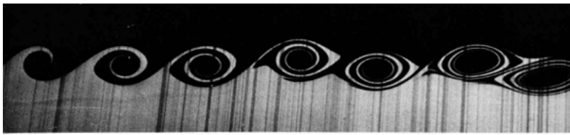
Figure 1.4: Kelvin-Helmholtz instability arising from two layers of water with different velocities, being the upper one the fastest. Adopted from [7].
