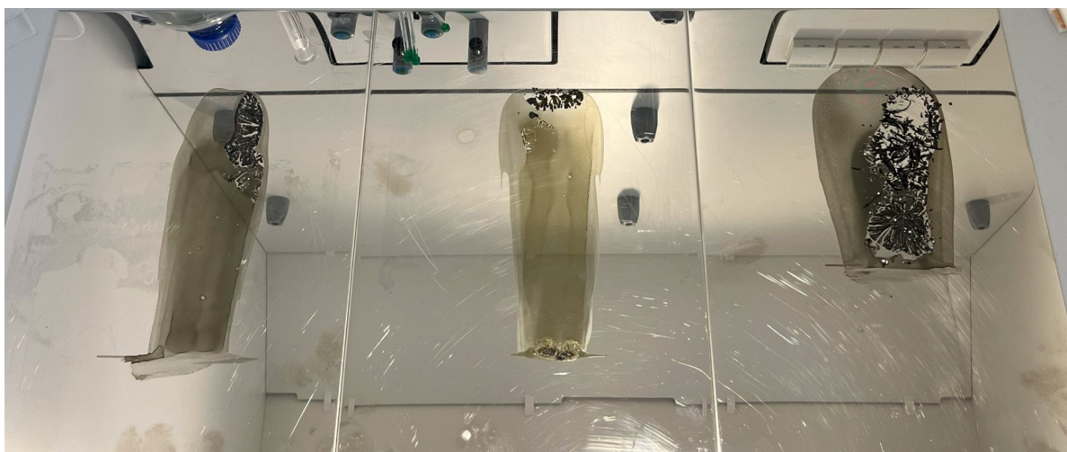
Figure B.2: First batch of membrane casting after oven treatment (from left to right: 0.5%, 1%, and 2% GO).
