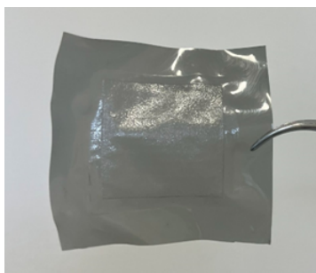
Figure D.20: Image of a swollen membrane post electrolyser.
