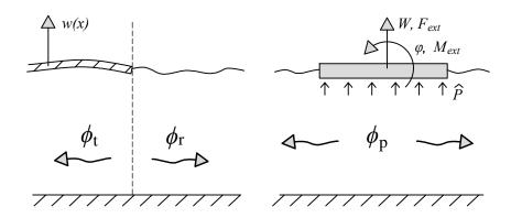
Figure 2: Excitation of the body generates waves (right image) which are party reflected and transmitted by the ice sheet (left image)
