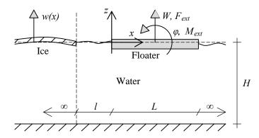
Figure 1: The waves generated by the body's motion reflect at the ice-open water interface. The pressure exerted by the reflected waves alter the body's response.
