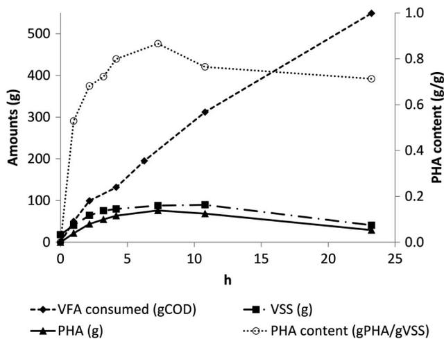
**Fig. 7.** Production of PHA-rich solids in the accumulation process; the lion's share of PHA was produced during the first 4 h (Day 9).
