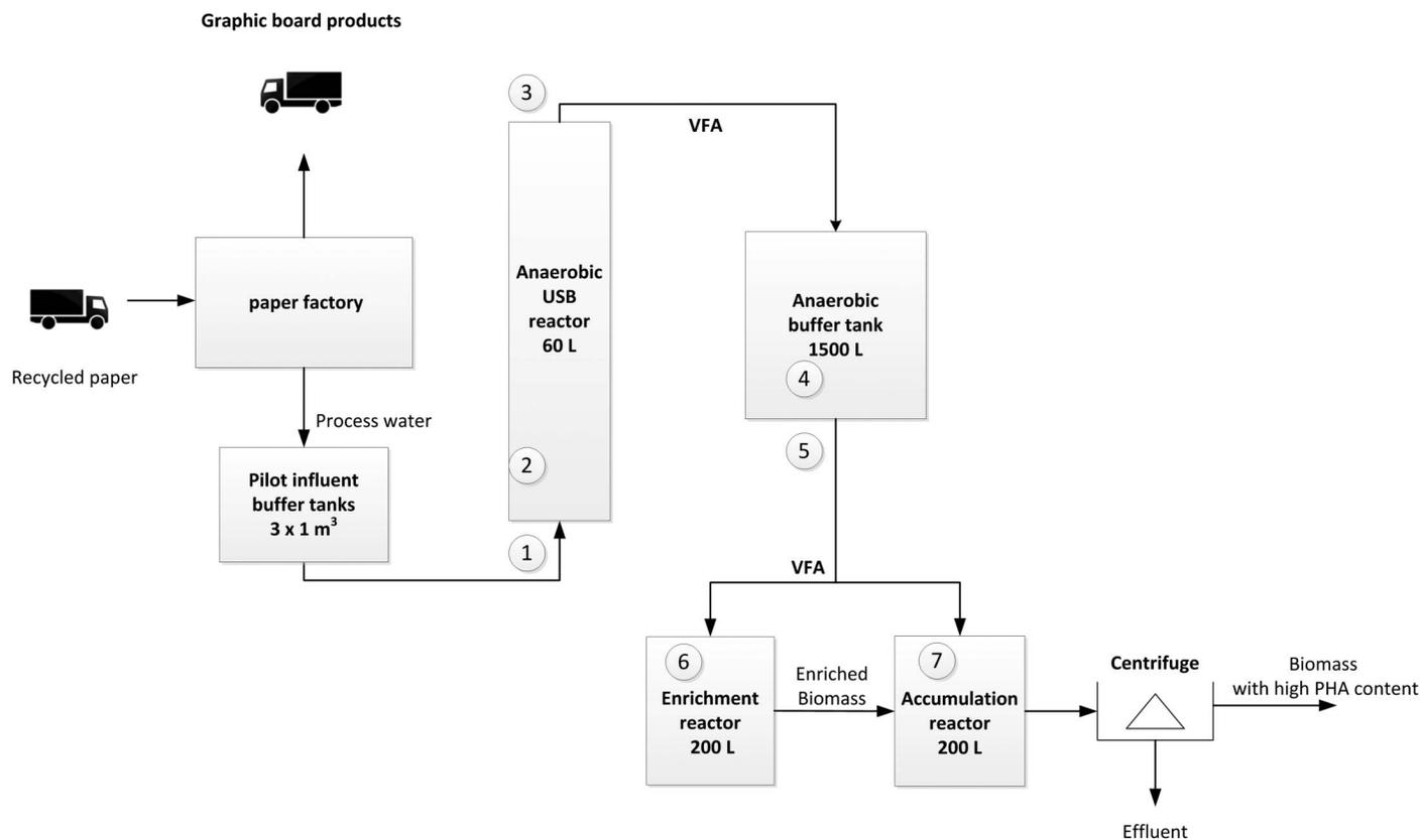
**Fig. 1.** Pilot system for PHA production from paper factory process water. The numbers indicate sample points. The unit operations in Sample Points 1–5 are related to anaerobic fermentation. Sample Point 6 is in the enrichment reactor and Sample Point 7 in the accumulation reactor.
