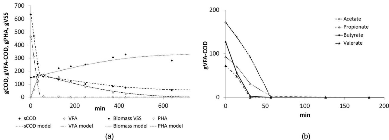
**Fig. 5.** Detailed characterization of a typical SBR cycle including (a) total amounts of VFA, PHA, and active biomass ( $X = VSS - PHA$ ); and (b) amounts of individual VFAs. Due to changing liquid volumes during the reactor feeding, data are represented as amounts and not as concentrations.
