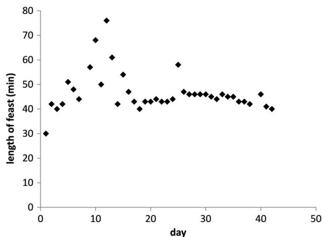
**Fig. 4.** Development of the length of the feast phase in the enrichment reactor evolving over consecutive cycles. The length of the feast phase was determined from the DO concentration profile, with the feast phase characterized by relatively low DO concentrations due to rapid substrate conversion (see also Fig. 3).
