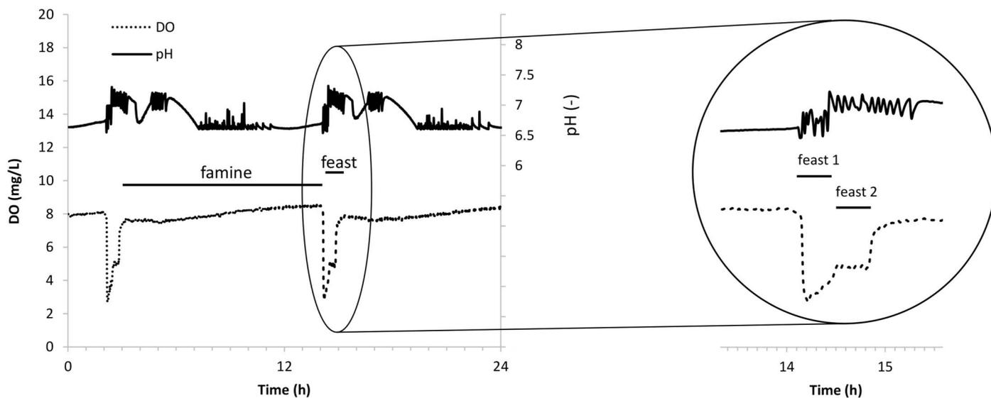
**Fig. 3.** Typical DO concentration and pH profiles during a period of two cycles ( $2 \times 12$  h) in the enrichment reactor.
