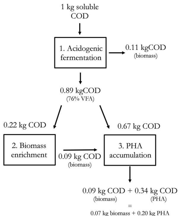
**Fig. 8.** Flow of COD in the PHA production process. The COD of biomass and PHA in this study were around 1.4 and 1.7 g COD/g, respectively.
