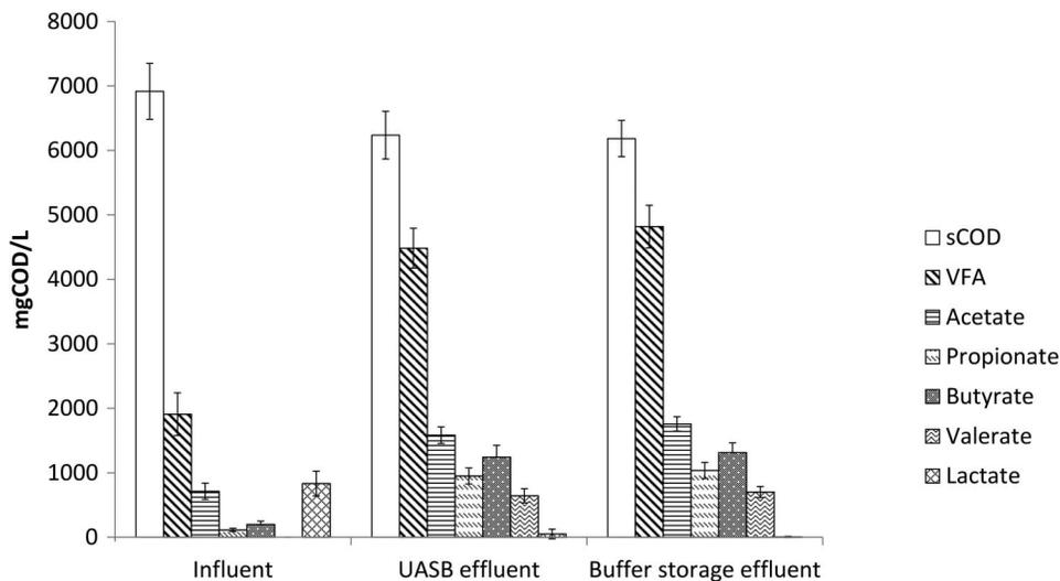
**Fig. 2.** Composition of the VFA fraction in the influent and the fermented process water. Error bars represent the standard deviation over the data set ( $n = 42$ ).
