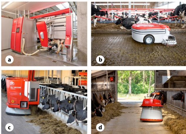
Figure 1: a) Lely Astronaut, the milking robot; b) Lely Collector, the manure cleaning robot; c) Lely Vector, the feeding robot; d) Lely Juno, the automatic feed pusher (courtesy of Lely)
