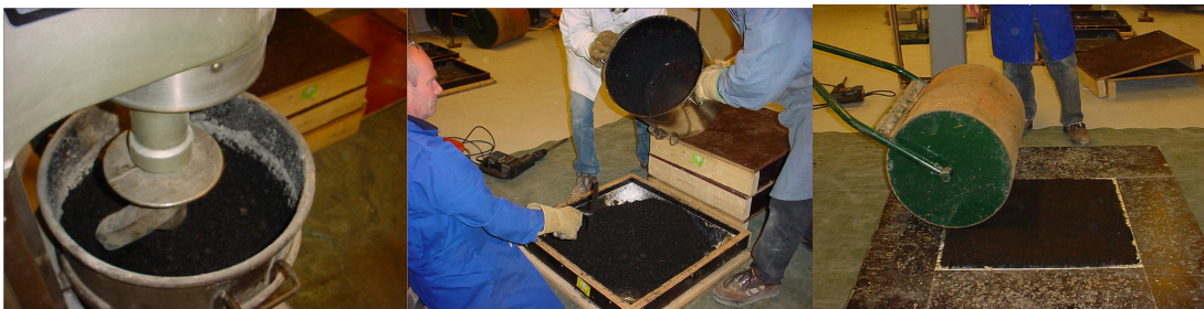
Figure 4.2: Mixing and pouring of porous asphalt mixture during slab preparation
