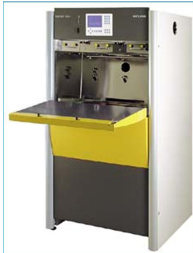
Figure 4.4: The SUNTEST XXL+ weathering instrument used for aging asphalt specimens
