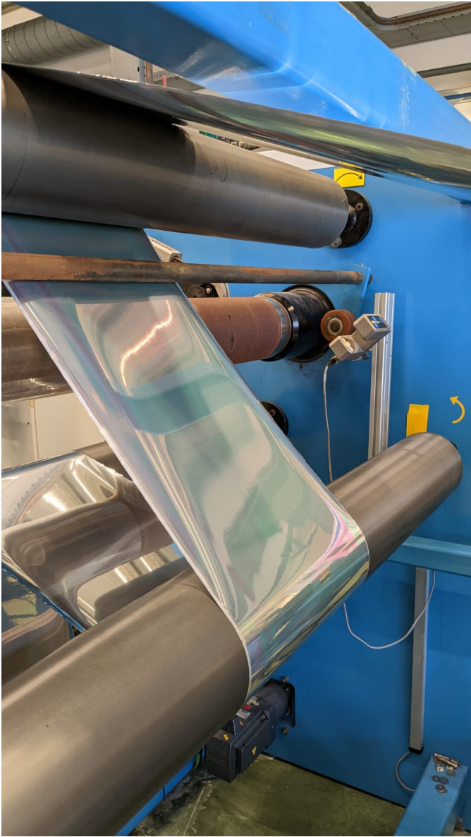
(a) Homogeneous thickness - TCO without striping
