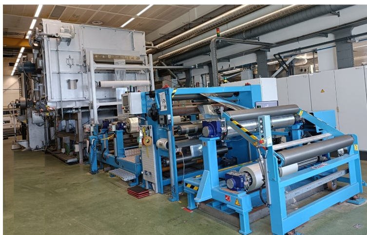
Figure 14: Experimental setup of the production APCVD machine
