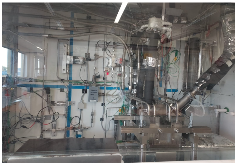
Figure 19: Experimental setup of the lab scale research APCVD tool
