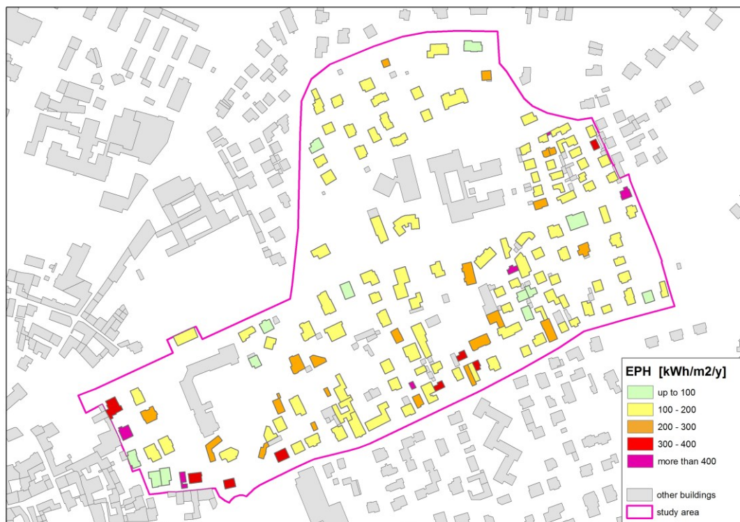
Figure 13. Estimated energy consumption for the retrofitting scenario “Roof insulation”. Image source: authors.
