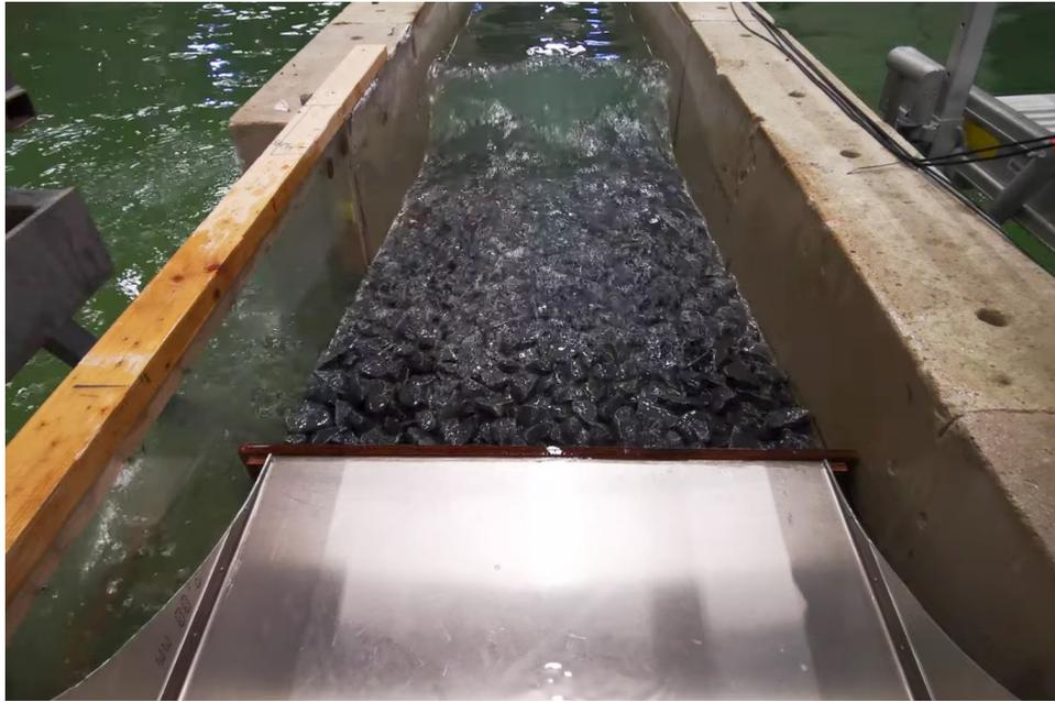
**Figure F.7:** Picture of a breaking wave on the slope of the breakwater with  $\cot \alpha = 6$
