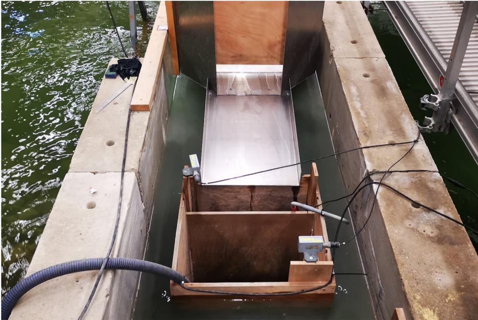
**Figure F.5:** Picture of the chute and the overtopping box at the back of the model setup.
