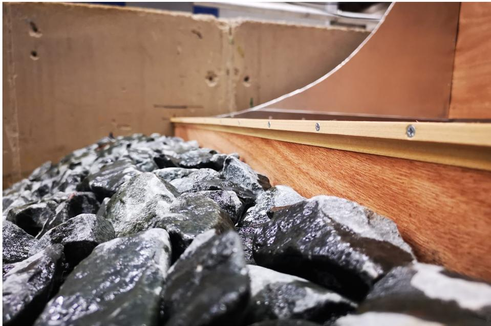
**Figure F.8:** Picture of the bull nose that was attached to the 5 cm crest wall
