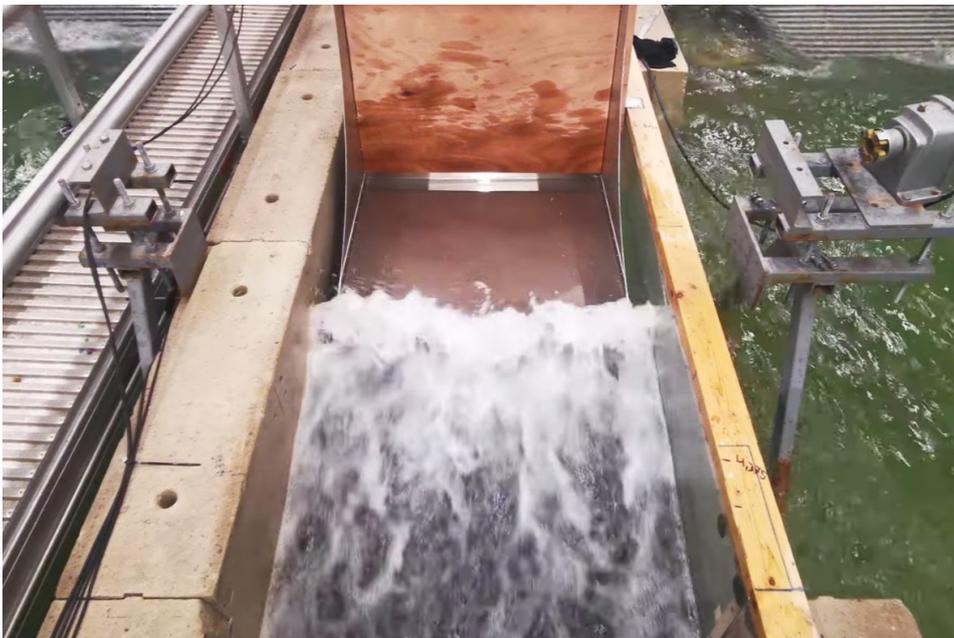
**Figure F.6:** Picture of wave overtopping at the crest wall.
