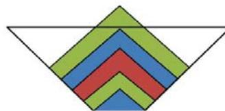
Figure 126: The Tepee filled with batch filling method
