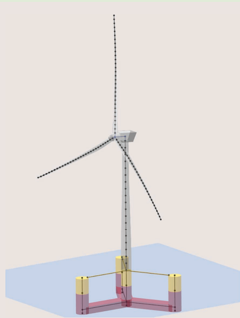
FIGURE S5 A representation of a floating wind turbine with beam elements connected in a multibody formulation.
