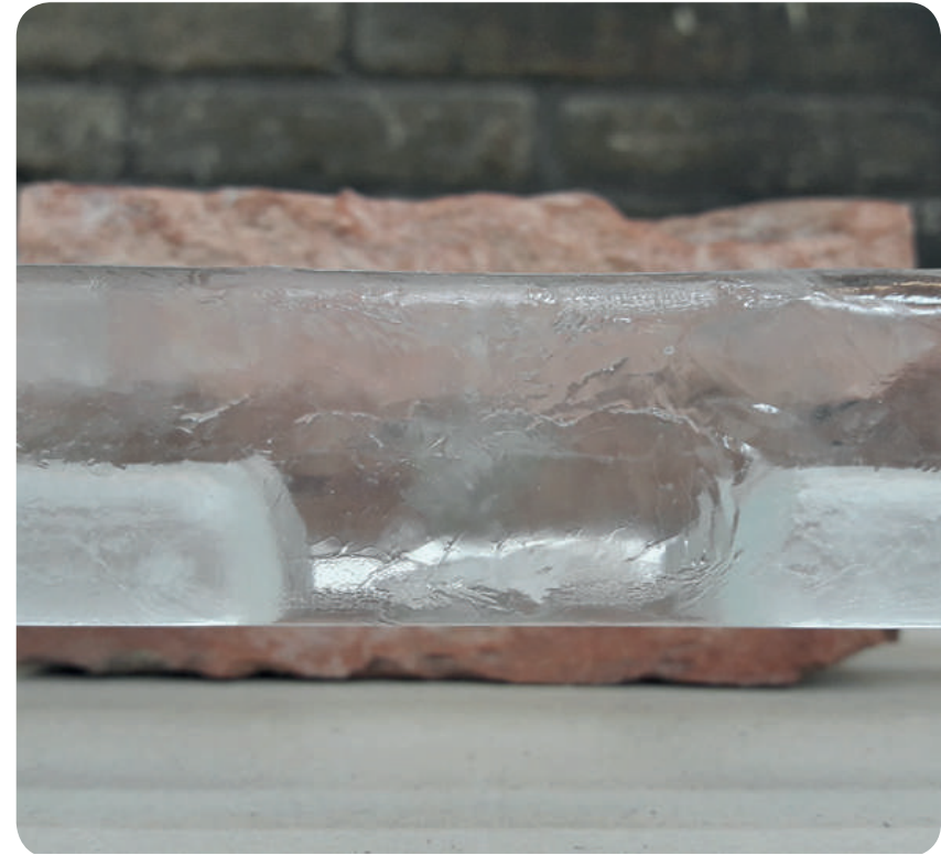
CAST GLASS SPECIMEN WITH A MORE TRANSPARENT APPEARANCE AND A GLOSSY SURFACE
