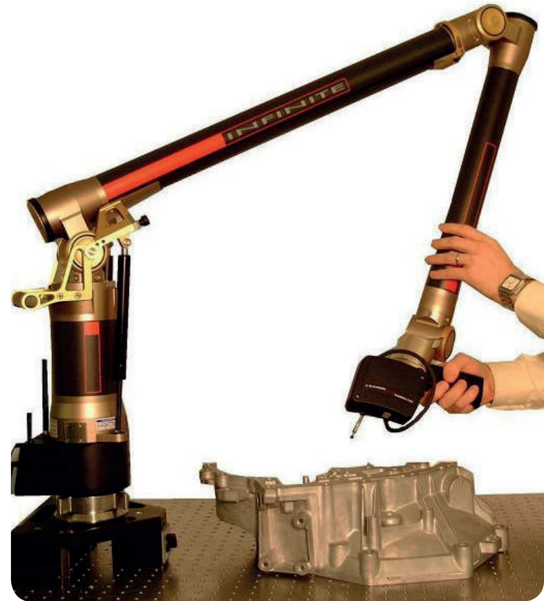
EXAMPLE OF A CONTACT SCANNER WHICH IS USED TO DOCUMENT THE SHAPE OF A STEEL ELEMENT.
