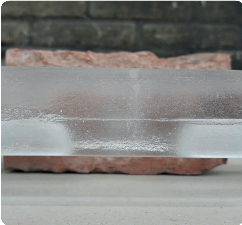
CAST GLASS SPECIMEN WITH A TRANSLUCENT APPEARANCE AND ROUGH SURFACE
