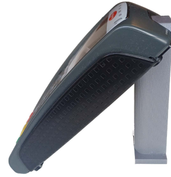
Fig. 3. The PoS iPP320 shown in the 45° setup. In the figure, we can observe the stand that we designed and 3D printed to keep the PoS in the correct position.
