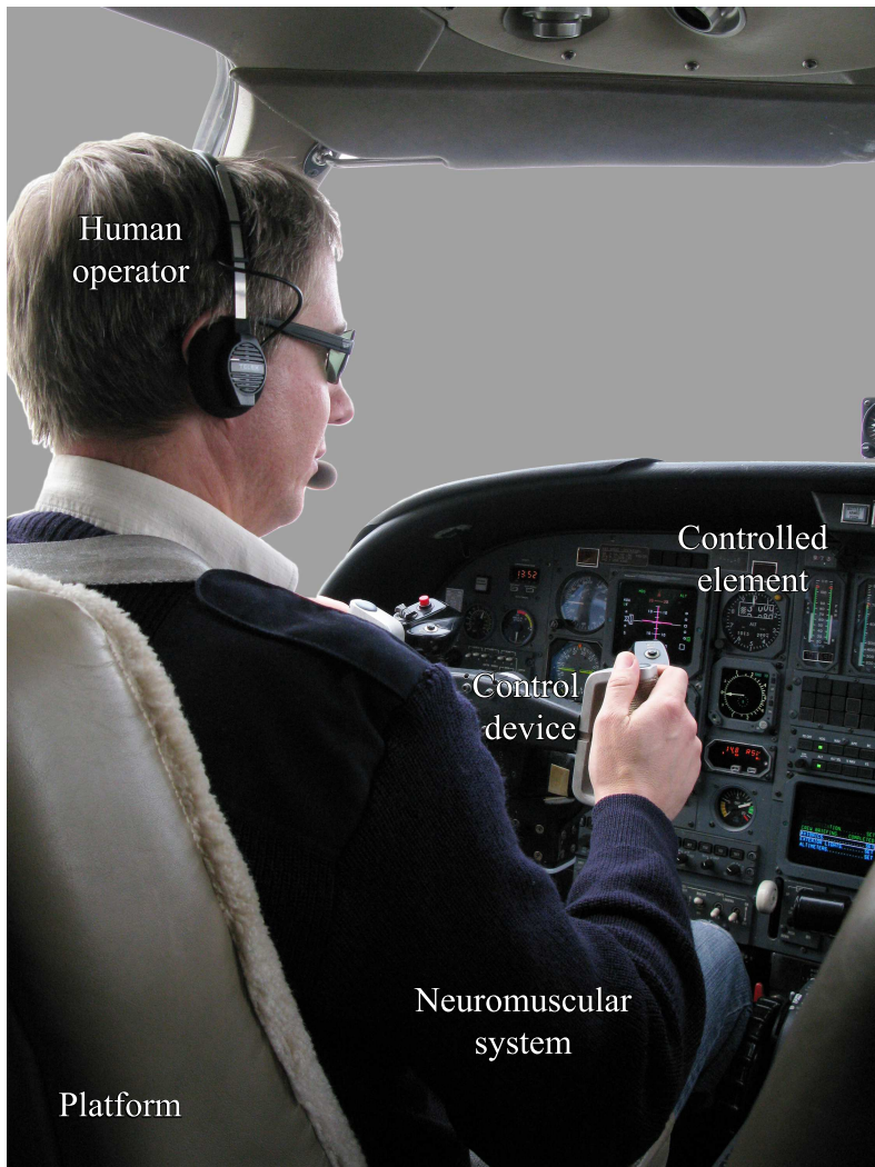
Figure 1.1: An example of a BDFT situation: an aircraft flying through turbulence. The pilot (human operator, HO) is controlling the aircraft (controlled element, CE) by means of the control column (control device, CD). The accelerations of the pilot's seat (platform, PLF) are transferred into the pilot's body (neuromuscular system, NMS). The involuntary motions of the pilot's arms result in involuntary control inputs.
