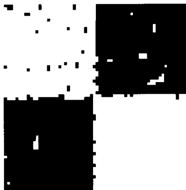
Figure 5.30: Thresholding result of the block composition of texture pair d57 and d92 at level 6 of the pyramid.
