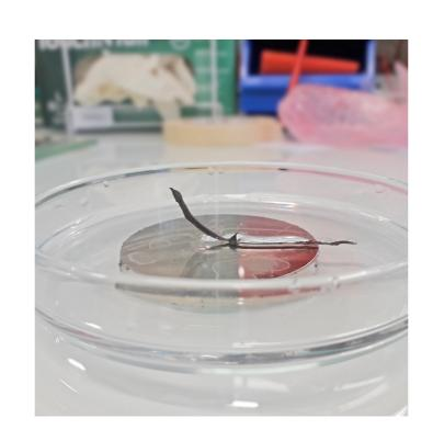
In one part of this project, the development of the ink recipe of silicones and magnetic particles, and a 3D printer with an electromagnet attached to the nozzle was started. This resulted in a proof of principle that can move and transform its shape in a magnetic field (see the figures at the left). This demonstrates the feasibility of fabricating magnetic soft materials at the faculty
