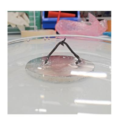
Magnetic soft materials consist of silicone with incorporated magnetic particles. The particles lay in magnetization patterns due to being printed under a magnetic field that rotates them, creating local North and South poles (see the figure above). During the shape transformation, the magnetic fields of these particles align with the external magnetic field, pulling the silicone in the programmed shape.
