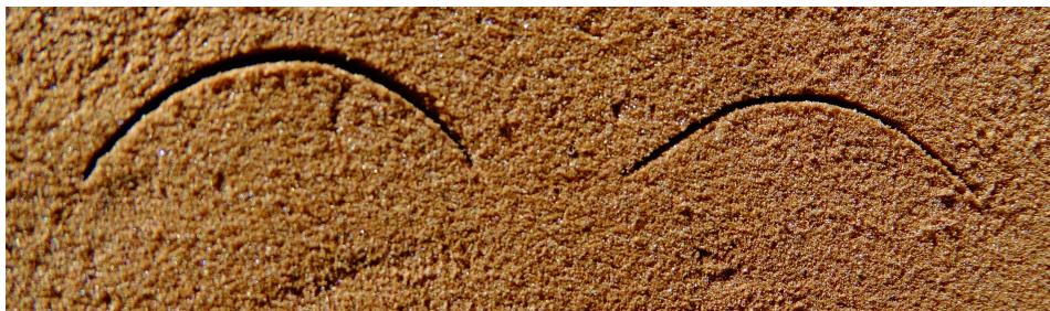
Figure E.5: Cross-section imprint in floral foam of the tape-measure after rolling (left) and before rolling (right) in the rolamite.
