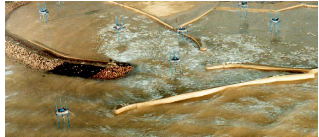
Fig. 22b West Harbour, Hartlepool, under 1:50 year storm, physical model
