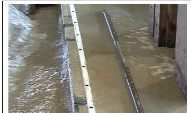
Figure 27 Observations of overtopping velocities and secondary wall loads
