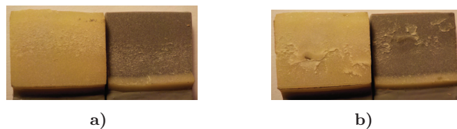
Figure 4.37: Fracture surfaces for test series SLJ2_A_1MPa tested at BAM.
