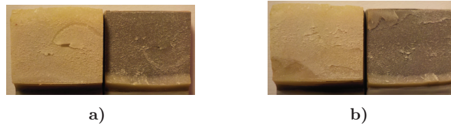
Figure 4.32: Fracture surfaces for reference specimens SLJ_Ref2 tested at BAM.
