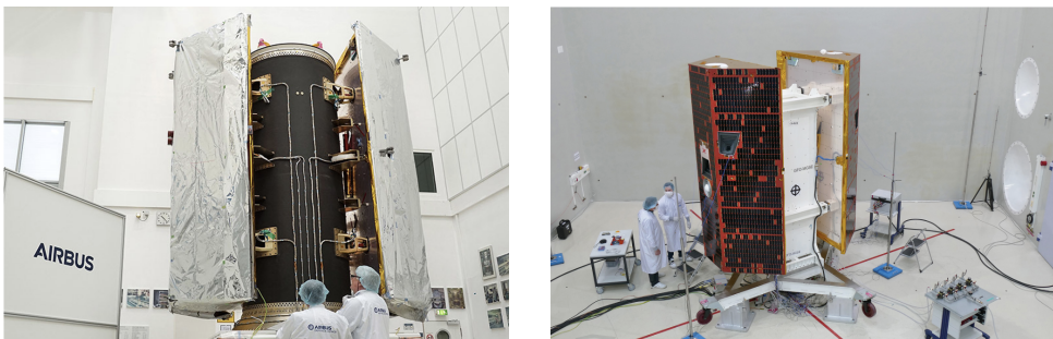
Figure 1.4: GRACE-FO twin satellites. Testing the dispenser structure (left). Source NASA . Preparations for the acoustic noise test (right). Source: AIRBUS .
