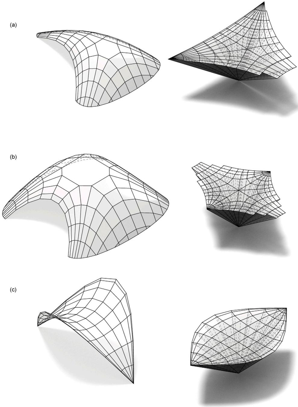
**Fig. 9.** Discretized analytical self-Airy shells and their Rankine diagrams. All self-Airy shells are drawn with the same  $b - y_0$  curve when  $b(0) = 1$  and  $b'(0) = 0$ . The  $a(x)$  curves are  $-\exp(x)$ ,  $-\cosh(x)$ , and  $\cos(x)$  in panels (a), (b), and (c) respectively.
