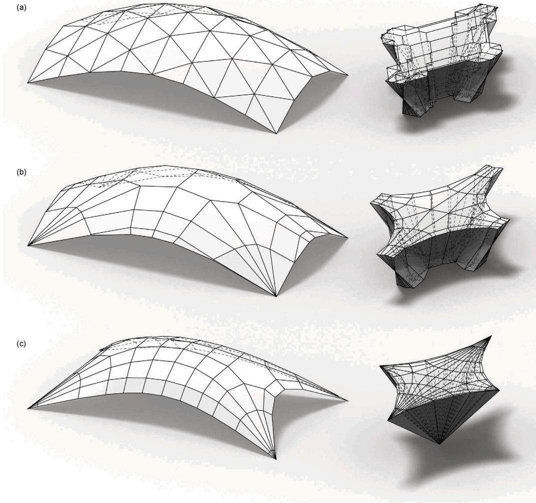
**Fig. 7.** Planar funicular gridshells and their Rankine diagrams. (a) A triangular gridshell. (b) A quadrilateral gridshell. Although discretized into different patterns, both (a) and (b) are based on a common membrane shell. (c) A self-Airy gridshell, which has distinctly curved free edges tangent to planes. (Vertical lines to  $z = \pm\infty$  are excluded for visual clarity).
