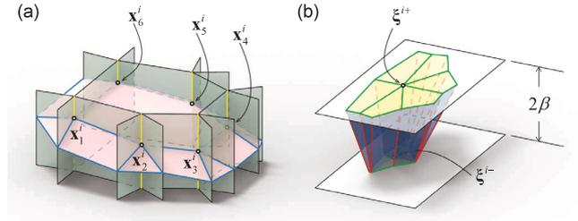
Fig. 5. A non-triangular gridshell (a) and its Rankine diagrams (b). The vertical loads (yellow lines) and the compression forces (blue lines) of the grids shells correspond to parallel faces (yellow) and lateral faces (blue) of the prismatoids. Prismatic cells above and below the hexagon  $x_1^i x_2^i \dots x_6^i$  correspond to vertices  $\xi^{i+}$  and  $\xi^{i-}$ , which connect 6 edges in the horizontal planes.
