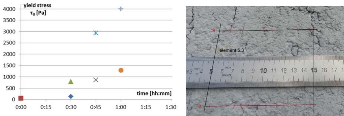
Figure 7 — Result of Element 5.3, deformed too late, at 1:00 h:mm. Left: the yield strength has increased quickly. Right: cracks are visible, comparable to the cracks generally caused by plastic shrinkage
