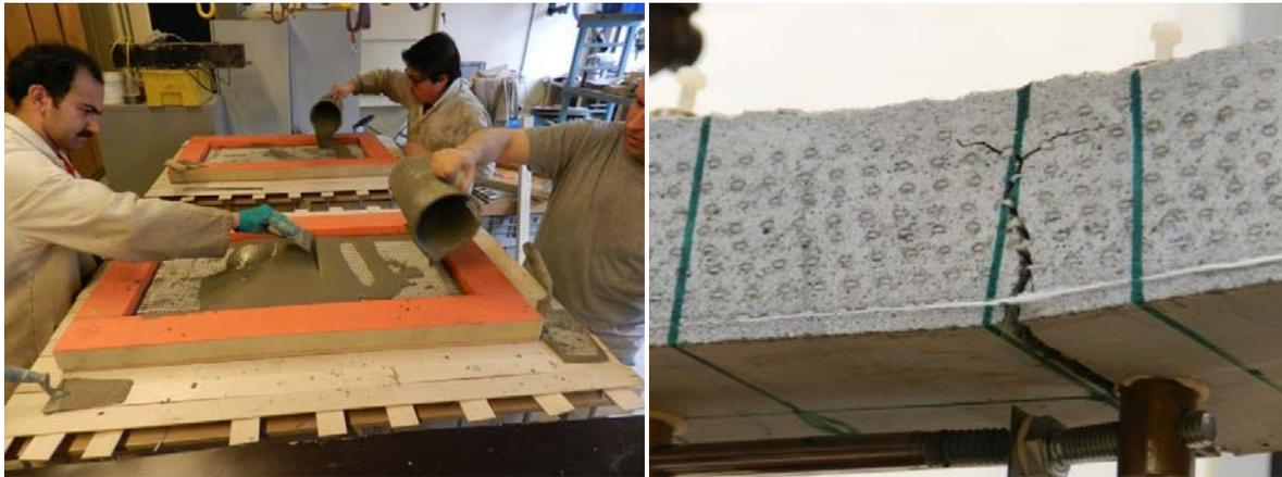
Figure 9 — Left: Production of the textile-reinforced elements according to the manual lay-up ‘lasagna’ method; right: 4-point bending test on 50 mm thick textile-reinforced concrete element.
