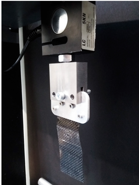
(b) The sample was connected to the load cell with 5 kN capacity for the measurements with glass substrates.
