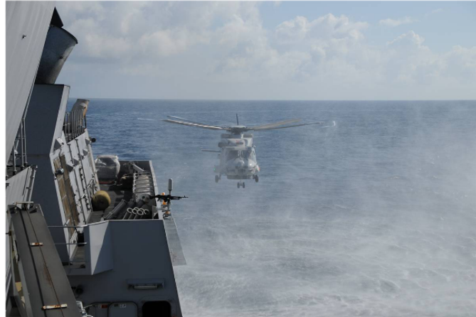
Figure 2.8: Sea spray originating from the main rotor downwash [12]
