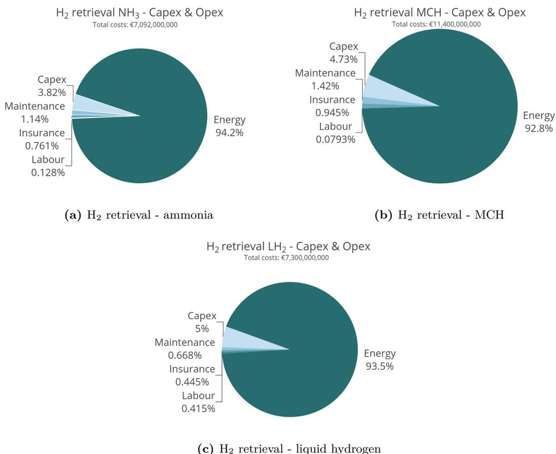
**Figure 5.5:** All the contributed costs of the H<sub>2</sub> retrieval for all carriers, based on the model output
