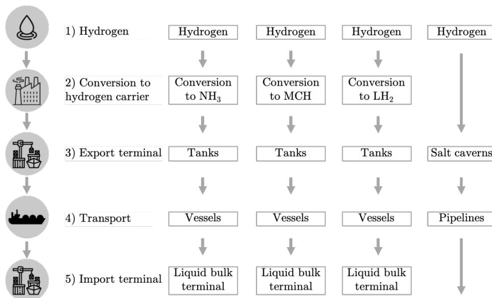
**Figure 2.7:** Supply chain of the different hydrogen carriers
