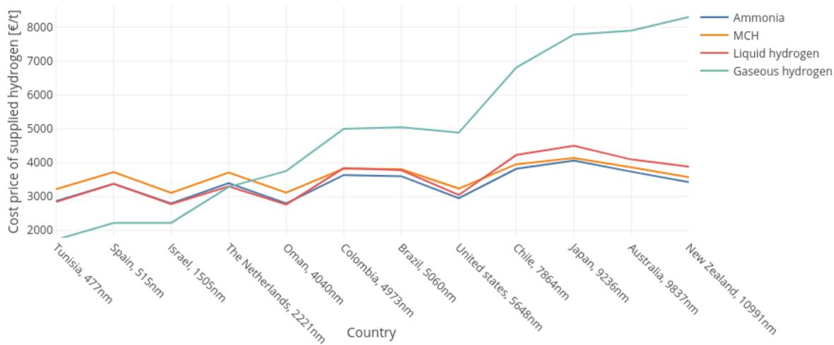
**Figure F0.6:** Cost price of the supplied hydrogen for the import in Italy varying with the countries, with a demand of 700,000 t/y
