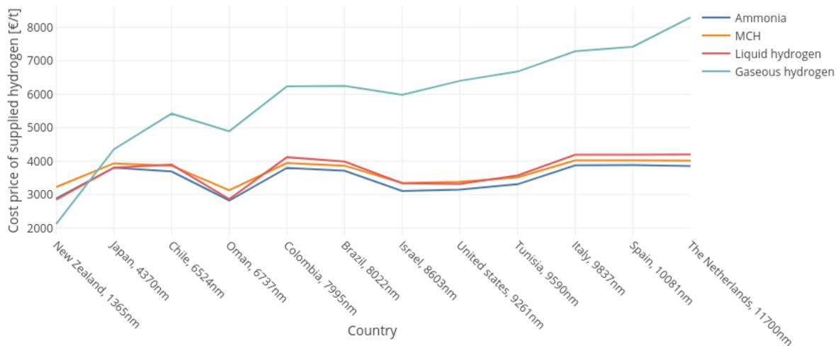
**Figure F0.1:** Cost price of the supplied hydrogen for the import in Australia varying with the countries, with a demand of 700,000 t/y
