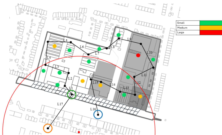
Figure 3.4: The concluded configuration of the 5GDHN and its additional components on the Werf [5]
