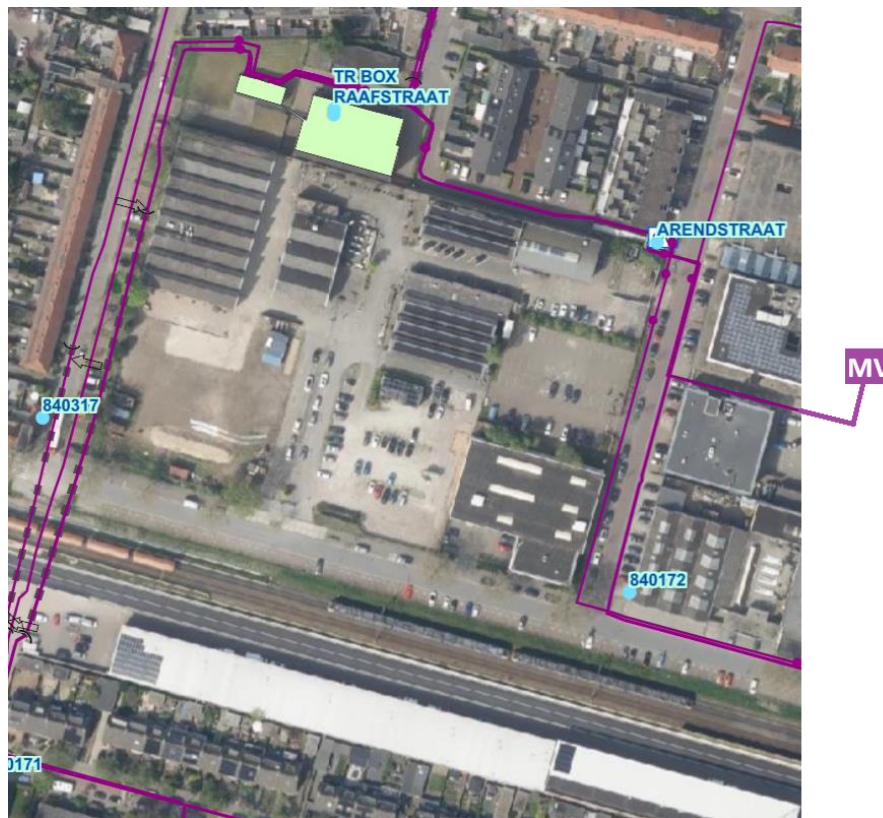
Figure 3.8: The medium voltage infrastructure layout on the Werf as supplied by the DSO
