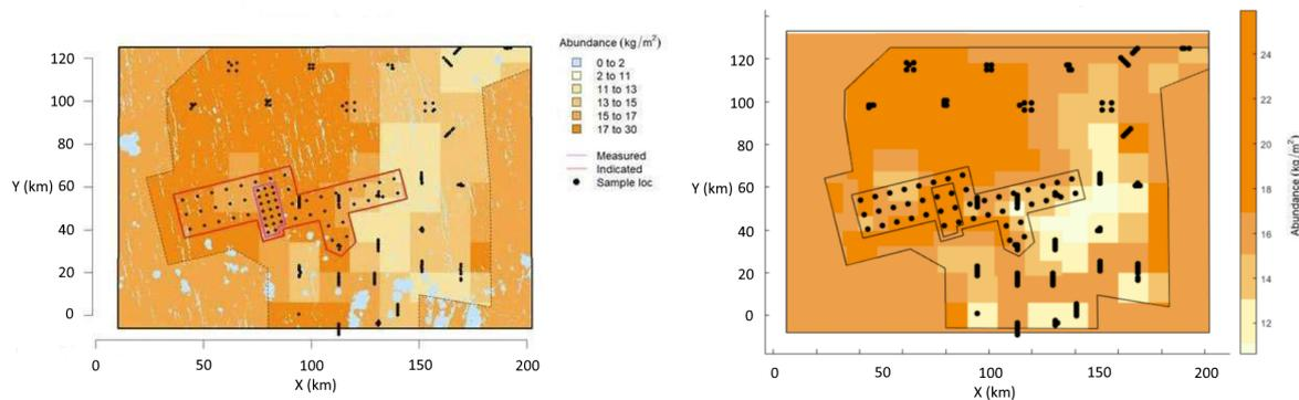
Figure 4.3: A visual comparison between the resource assessment of the technical report (left) and the recreation of the same block model for the purposes of this thesis (right). Black dots are sample locations. In the left figure the different resource classification levels are indicated with coloured polygons. Purple for measured resource, red for indicated resources. The black polygon shows the interpolation limit, outside of that the nodule abundance was set to the mean.
