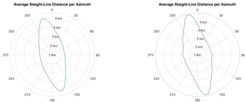
Figure 4.10: Two rose diagrams showing the average SLD for each azimuth for site 3. On the left, the rose diagram for site 3 includes a hard-constraint for the nodule types. On the right, the rose diagram assumes that all nodule types are traversable.
