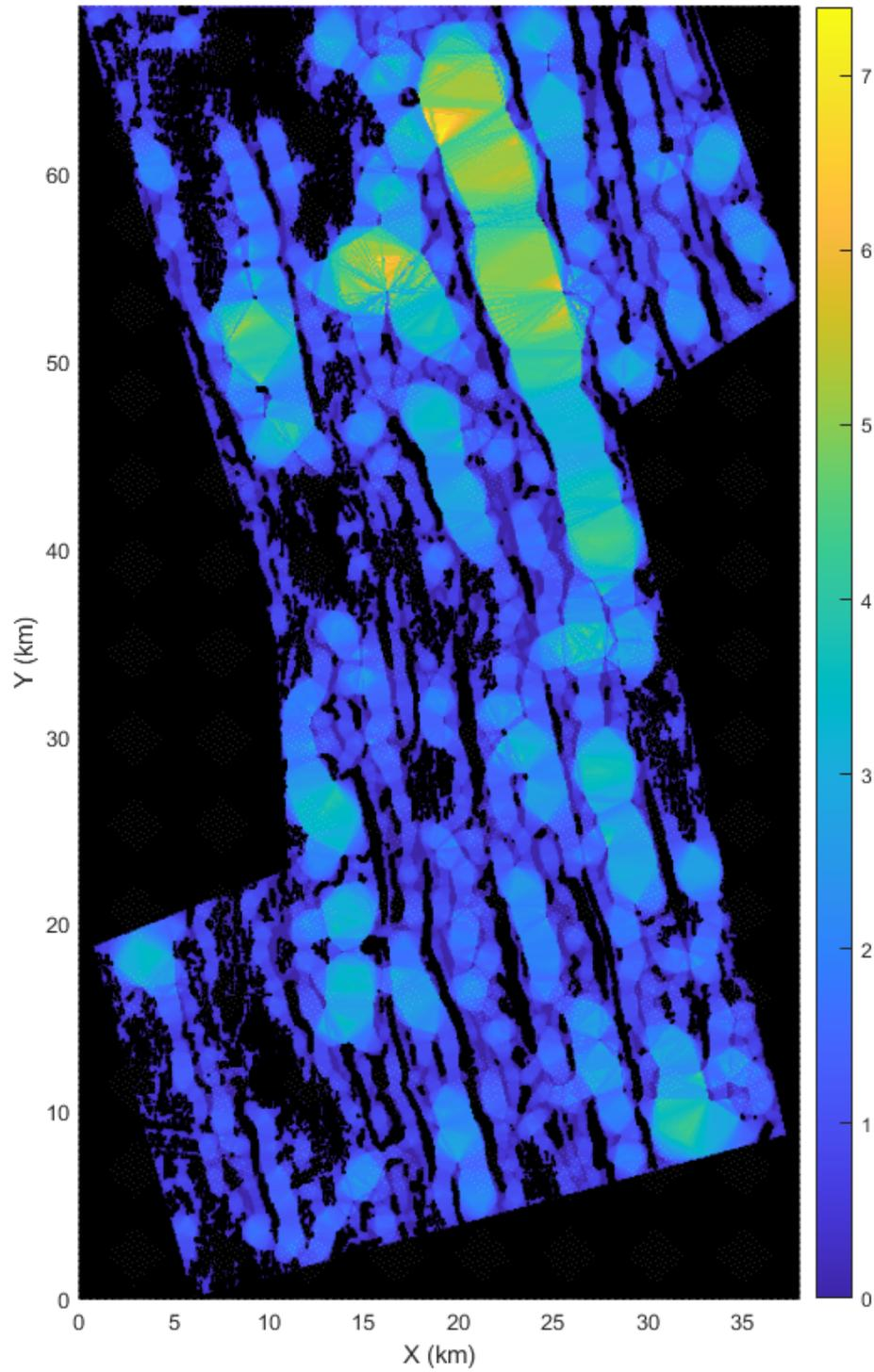
Figure B.3: The minimum SLD for site 3. The constrained pixels include slope constraints and nodule type constraints, shown in figure 4.8.
