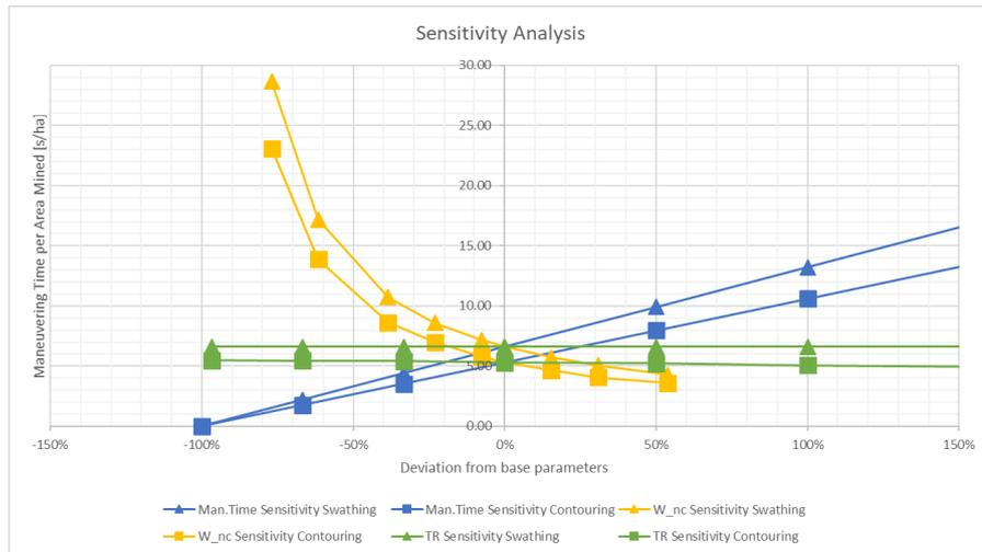
Figure 7.8: The sensitivity of the three parameters on the added maneuvering time per area mined. The base parameters are listed in table 5.1.
