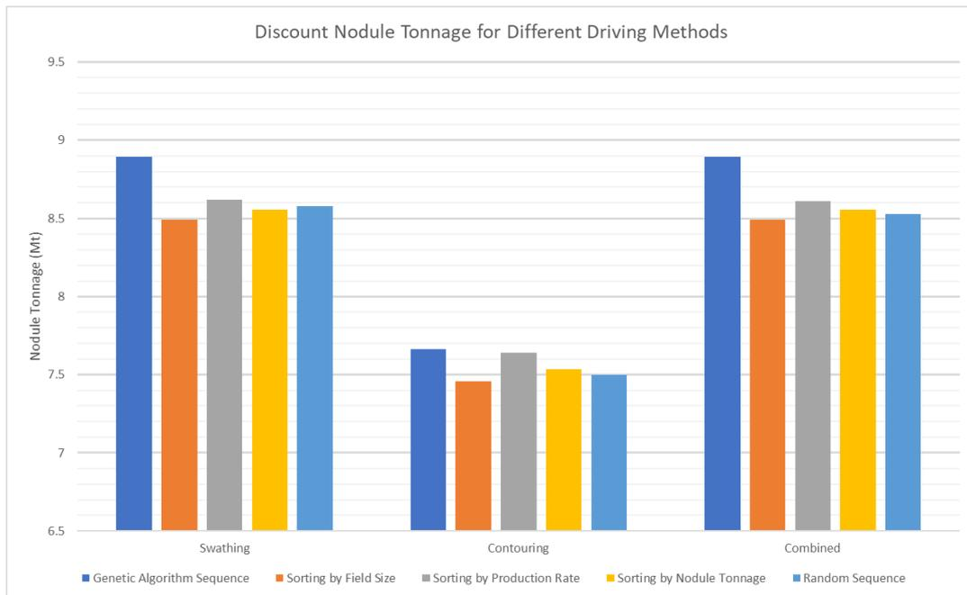
Figure 8.3: Discounted Nodule Tonnage for the different sequences of fields and different driving methods.
