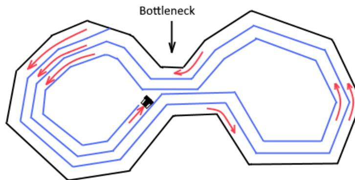
Figure 7.5: A schematic illustration of a field with a bottleneck. The nodule collector runs into its own track on the third loop.
