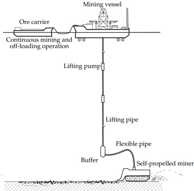
Figure 1.2: Mining concept. Adapted from Lee et al. [2012].
