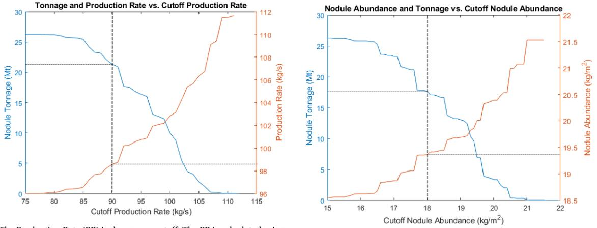
(a) The Production Rate (PR) is shown as a cutoff. The PR is calculated using equation 5.6, nodule abundance from kriging, and input parameters from table 5.1.
