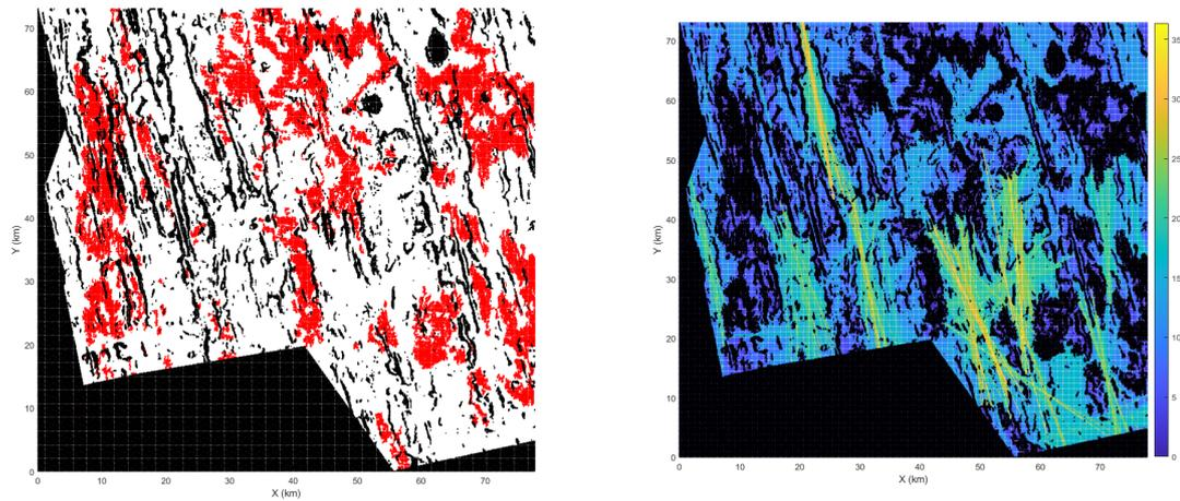
Figure B.7: On the left the constrained areas of site 5. Nodule type 2 & 3 indicated in red. Boundaries and slopes above threshold in black. On the right the maximum SLD
