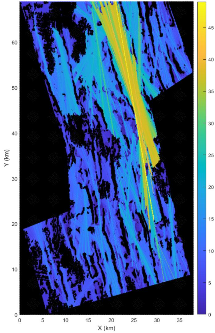
Figure B.1: The maximum SLD for site 3. The constrained pixels include slope constraints and nodule type constraints, shown in figure 4.8.
