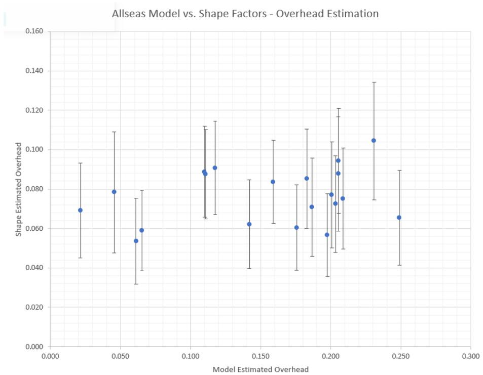
Figure 6.4: The overhead (percentage of unproductive time) as estimated from the shape indices (Y-axis) is plotted against the overhead found by the simulation (X-axis).
