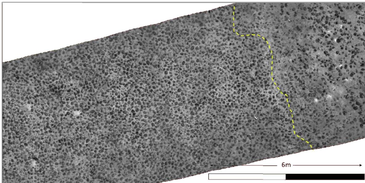
Figure 2.3: Photographs from the seafloor made by a UAV traverse. The dashed line indicates a change from nodule facies type 2 (left) to nodule facies type 3 (right). From AMC [2019].
