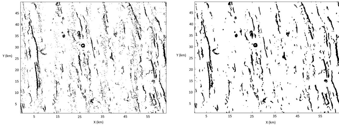
Figure 4.4: Cutout of a smaller area. Black pixels indicate areas with a slope that exceeds the  $8^\circ$  threshold. On the left the unfiltered area. On the right the neighborhood filter is applied. Vertical bands of pixels that are perceived as noise have been removed. Areas with a high density of black areas have been joined together.
