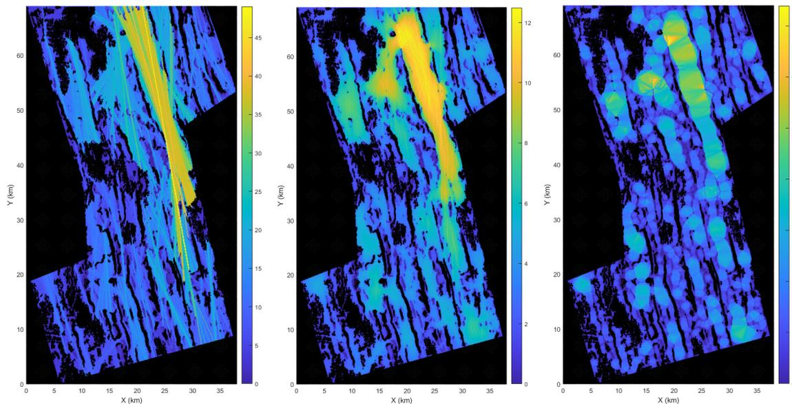
Figure 4.9: The maximum SLD (left), the mean SLD (middle), and minimum SLD (right) in each direction. Distances in kilometers. A larger version of the same plots can be found in the appendix figures B.1 to B.3.
