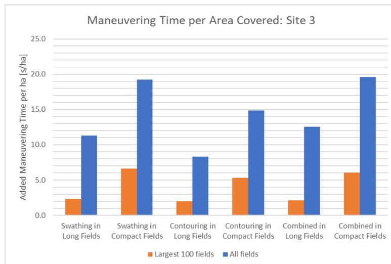
Figure 7.6: Maneuvering time per hectare for two sets of fields in site 3: long and compact fields. Three types of driving pattern are used: swathing, contouring and combined. Lastly, the production rates are compared between the largest 100 fields and all the fields combined (including the 100 largest).
