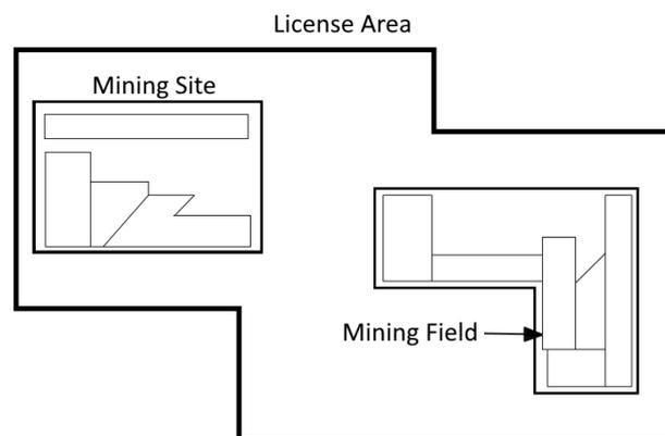
Figure 2.5: Schematic illustration of a deep-sea mine plan. After [Volkmann, 2018].
