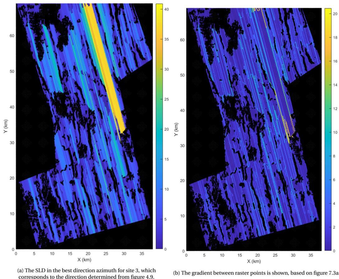
Figure 7.3: Site 3 is shown with hard constrained areas in black, previously shown in figure 4.8. The hard constrained areas correspond to the boundaries, slopes above thresholds, and nodule type 2 3.
