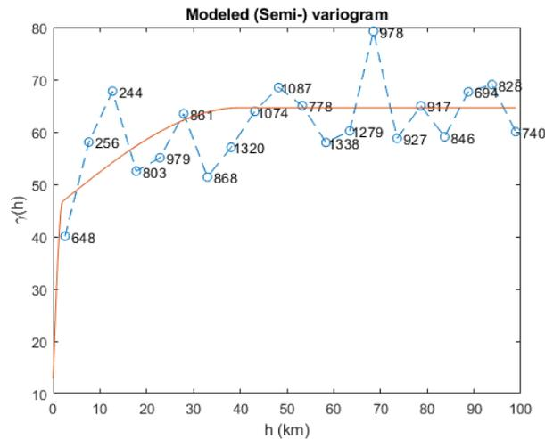
Figure 4.2: Omni-directional experimental variogram (blue) of NA samples. The fitted variogram model is indicated in red. The numbers indicate the number of data pairs used for that point. The variogram is not normalized. Variogram MATLAB function made by Schwanghart [2020].
