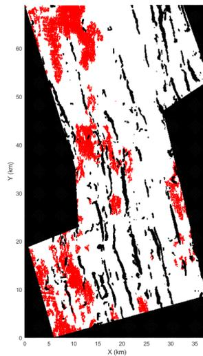
Figure 4.8: The constrained areas in site 3. Areas outside the boundaries of the site are shown in black. Areas that have a slope above the traversable threshold are also black. Areas with nodule types that are currently unmineable are indicated in red.
