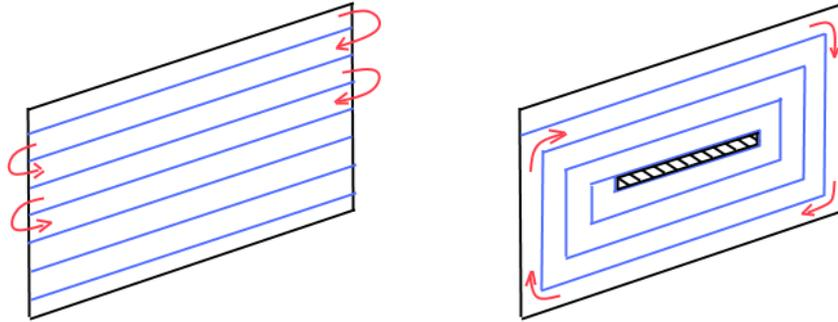
Figure 5.2: The same area covered using two different pathing patterns. On the left: swathing. On the right: contouring, which leaves a small part in the center of the field unmined. The patterns would be applied inside fields such as the ones indicated in figure 2.5.
