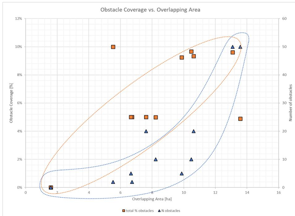
Figure 6.3: Results from the path planning model. Overlapped plotted against several obstacle parameters: area coverage of obstacles and number of obstacles. Note that the simulation without obstacles (Obstacle Coverage = 0%) overlaps for the two datasets.
