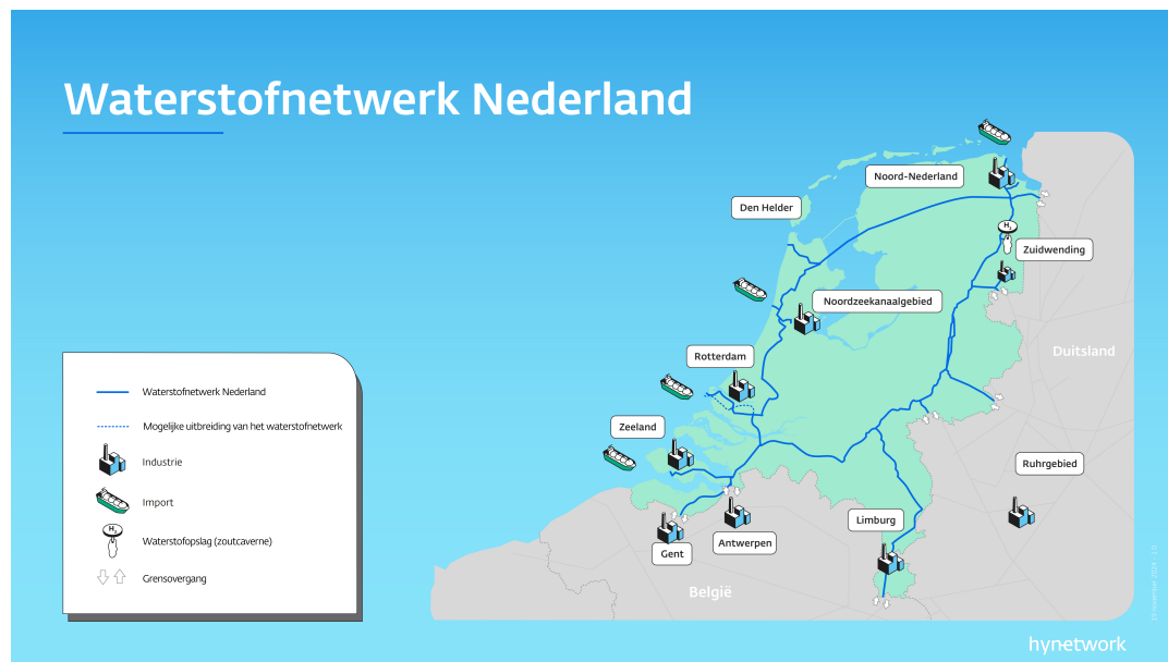
Figure 1.1: Overview of the planned national hydrogen network in the Netherlands, highlighting key industrial clusters, cross-border links, and strategic infrastructure nodes essential for enabling large-scale hydrogen transport and decarbonization.
