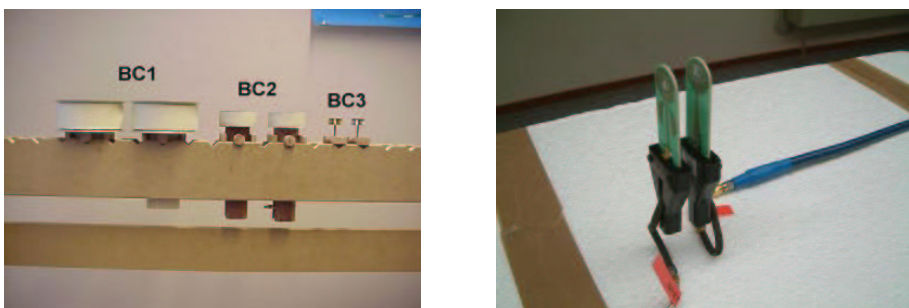
Figure 3.17: The bi-conical (BC) antennas (left) and Time Domain “Schantz” antennas (right).
