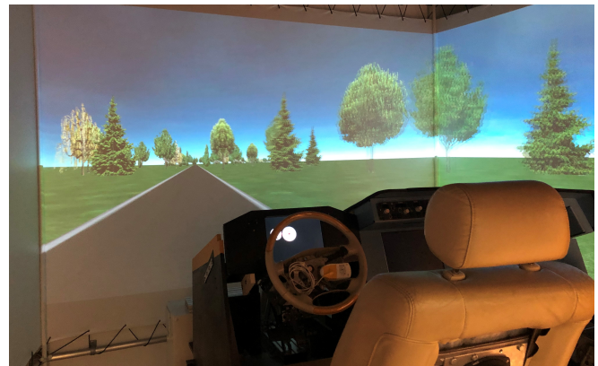
Fig. 5: Car simulation setup in the HMI-Lab fixed-base driving simulator.
