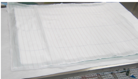
(e) Spreading of peel ply over the stacking
