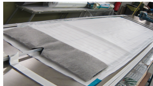
(f) Runner placed at the edge of infusion mesh
