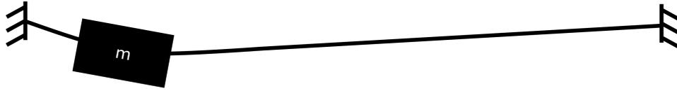
Figure 3.9: Exaggerated situation of deflection of the axis
