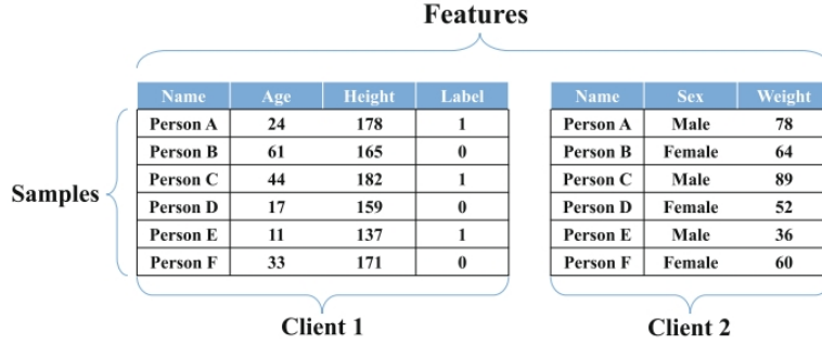
Figure 2.4: Features pace and samples space of Vertical Federated Learning . In VFL, every client has all the data samples, but each client has different features of these data, and only the guest party has the labels of these data. Here, Client 1 is the guest party and Client 2 is the host party [40].
