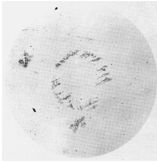
Figure 4.4 Scratches showing area with plastic deformation at sphere-sphere contact (from (Deresiewicz 1953))
