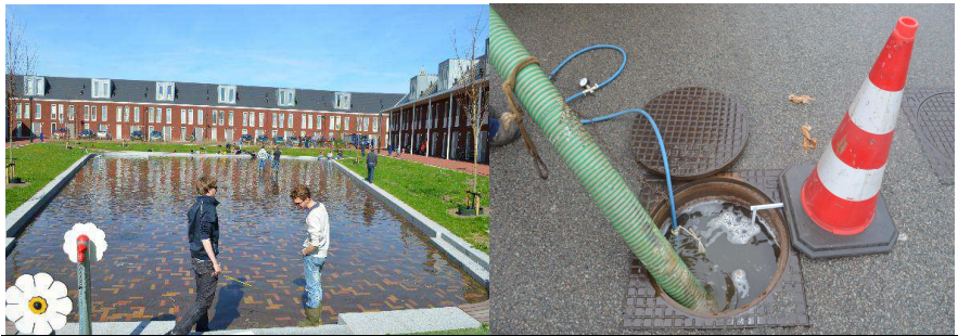
Figure 1-6 Full scale test at watersquare (left) and full scale test on filter drains (right).
