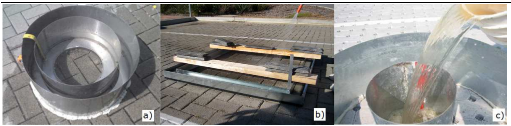
Figure 4-3 Modified Ring Infiltrimeters used for Permeable Pavement Testing (a) DRIT (Fassman & Blackbourn, 2010); (b) Square, Double Ring (Lucke & Beecham, 2011); (c) Single Ring Surface Inundation Test (Bean et al., 2004).
