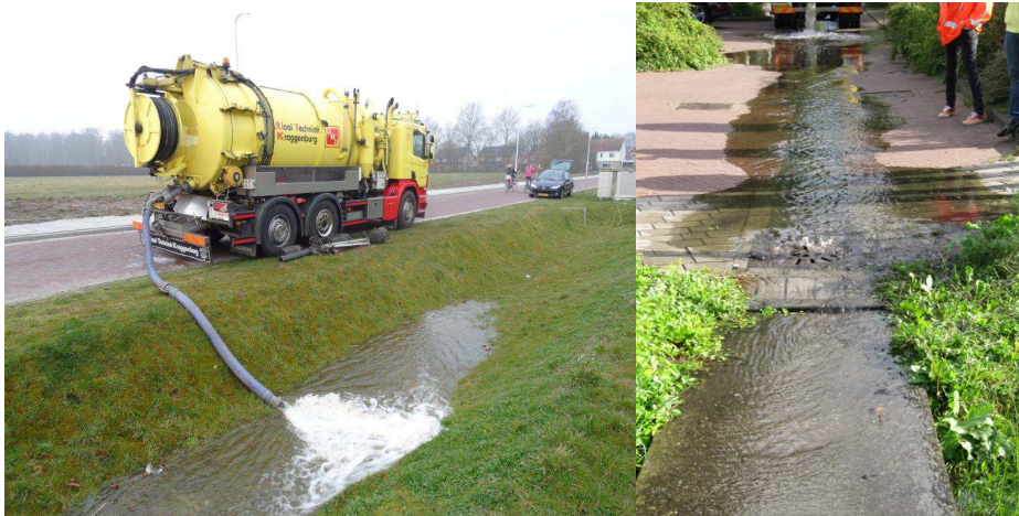
Figure 5-3 Full scale test for monitoring the hydraulic behaviour of swales
