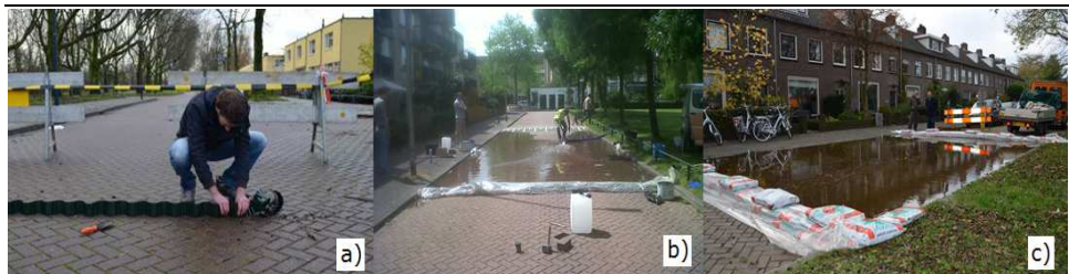
Figure 4-5 Various Dam Variations Used at the Different Test Locations (a) Impermeable barriers; (b) Plastic wrapped soil core; (c) Soil-filled plastic bags.
