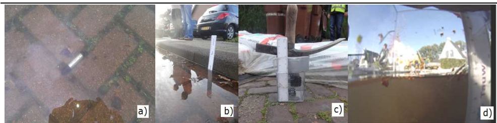
Figure 4-7(a) Minidiver installed at lowest point of pavement; (b) Hand measurement point; (c) Underwater camera set-up; (d) Underwater camera view.
