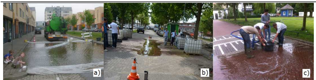
Figure 4-6(a) Water truck supply; (b) Water tank supply; (c) Pumping from canal.
