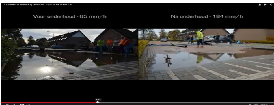
Figure 4-10 visualisation by timelapse camera showed the infiltration capacity before and after maintenance of permeable pavement at the same time on video. ( http://www.climatecan.nl/page?details=60 ).
