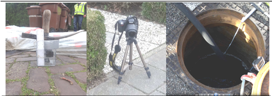
Figure 1-7 Underwater camera set-up at permeable pavenment (left), timelapse camera (middle), camera set up for monitoring infiltration transport drainage (right).
