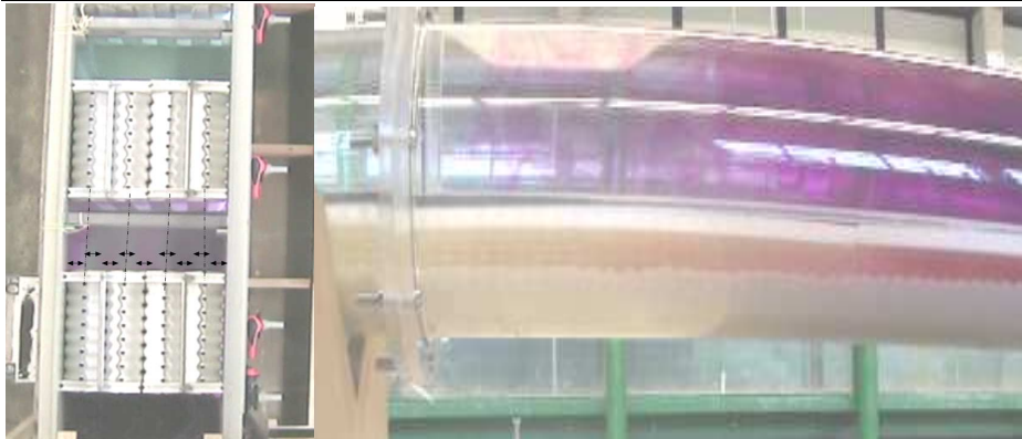
Figure 3-5 Visualization of preferential flow in lamella separator (divided in 9 parts where the upper 4 parts have no visual current due to the construction bars of the lamella at the dotted lines), Sedipipe (right) where the flow above the grid is dominant.
