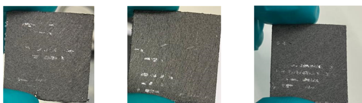
Figure 4.12: GDE back surface of three parallel samples with 2 mol/L KOH anolyte, at j=50 \text{ mA/cm}^2 , duration = 1h
