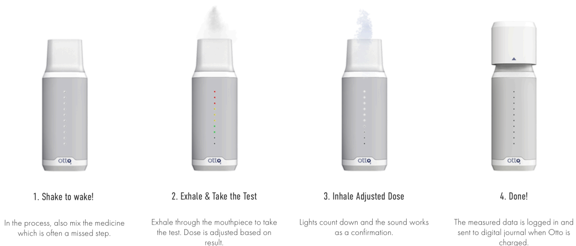
Figure 12: ‘Otto’ by Birnur Sahin (2020); a device to measure, track and inhale asthmatic medicine in the right way, guided by lights and sounds.
