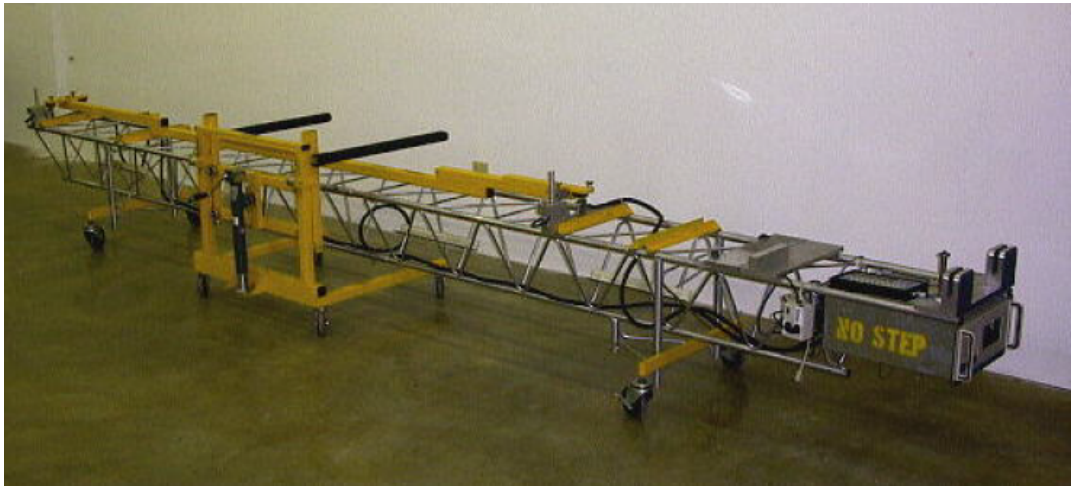
Figure 2.5: The USBF span moment measuring system used for static balancing developed by Avion services (Buckel (2003)).
