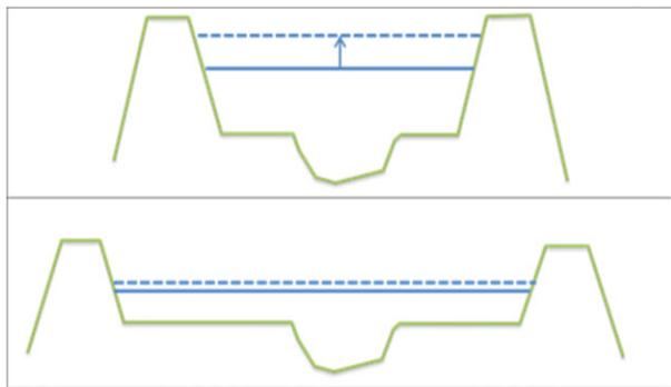
**FIGURE 1** Degree of water level rise with increasing river discharge in a river with a narrow cross section versus one with a wide cross section of equal capacity
