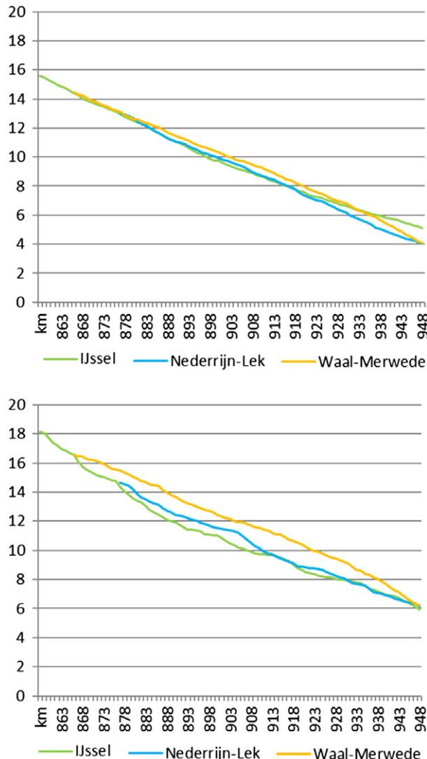
**FIGURE 5** Slope of the three Rhine River branches between the German–Dutch border and km 950 for a 1/10 (top) and 1/10,000 per year flood (bottom)
