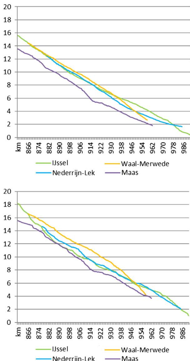
**FIGURE 6** Slope of the fully embanked lowland part of the Meuse River in comparison to the three Rhine River branches for a 1/10 (top) and 1/10,000 flood (bottom)
