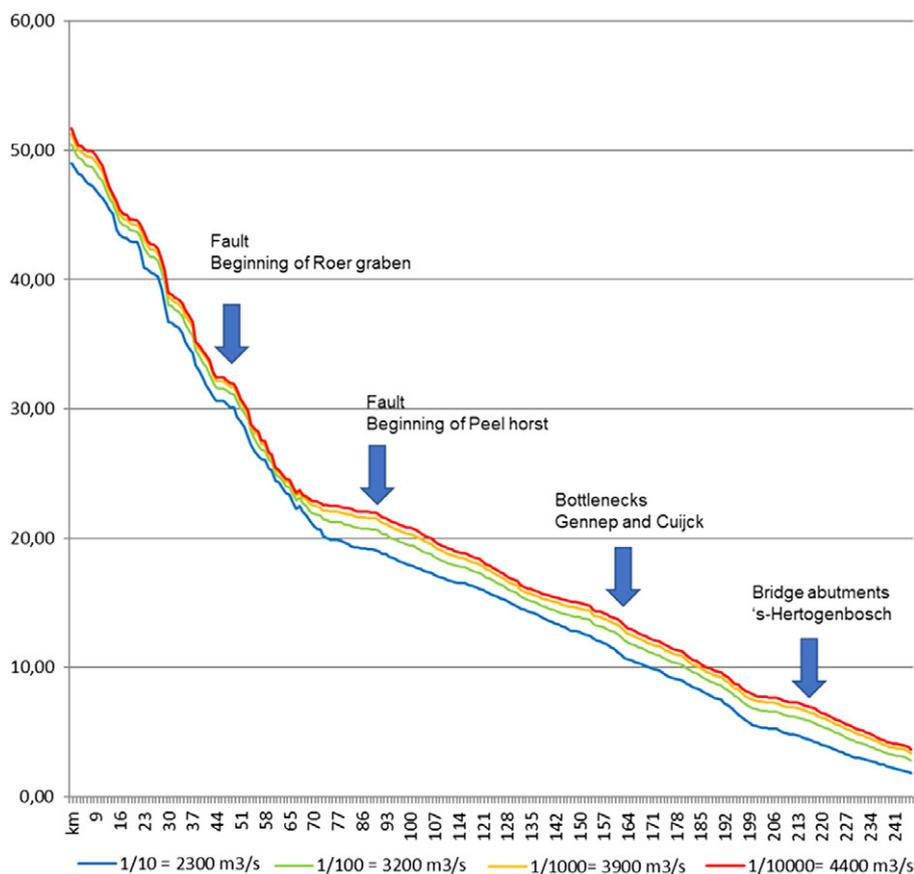
**FIGURE 3** Slope of the Meuse River at 4 successive flood stages, corresponding with about 1/10 to 1/10,000 per year discharges at Eijsden, showing distinct differences between the steep upper Meuse, the remainder of the Meuse Valley (until km 150) and the embanked lower Meuse
