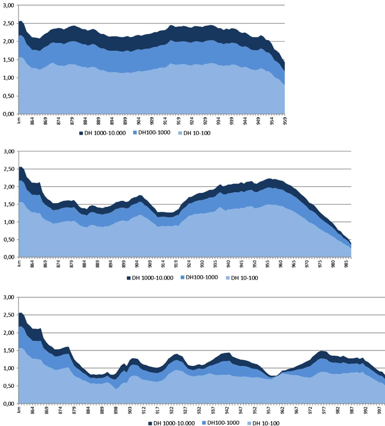
**FIGURE 7** Cumulative decimation heights for Bovenrijn-Waal (top), Bovenrijn-Nederrijn/Lek and Bovenrijn-IJssel (bottom). Mark that the rivers have different length (as loosely indicated by the different width of the graphs)
