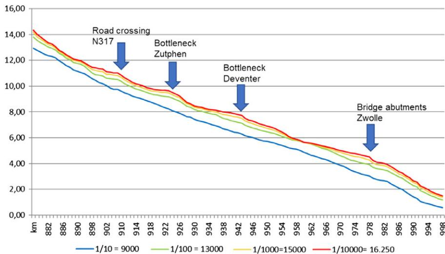
**FIGURE 2** Slope of the IJssel River at 4 successive flood stages, corresponding with about 1/10 to 1/10,000 per year discharges in the Rhine River at Lobith, showing increasingly marked set up of flood levels as caused by obstacles and urban bottlenecks
