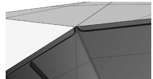
Figure 3.17 - seals curved upwards in the cornerpoints
