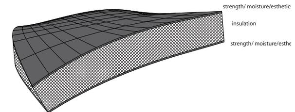
Figure 1.20 - combining functional layers in one sandwich element
