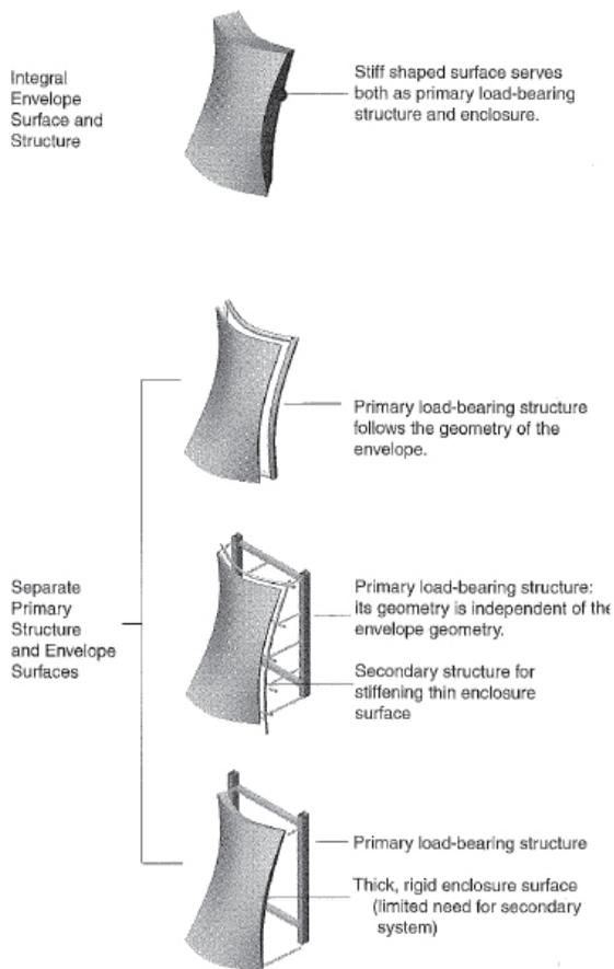
Figure 1.13 - Types of freeform building envelopes
