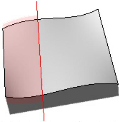
Figure 1.16 - CNC wire cutting, one dimensional path
