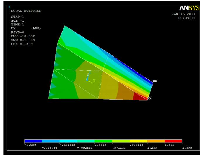
Figure 4.39 - normal stress in the face and deformation at the support
