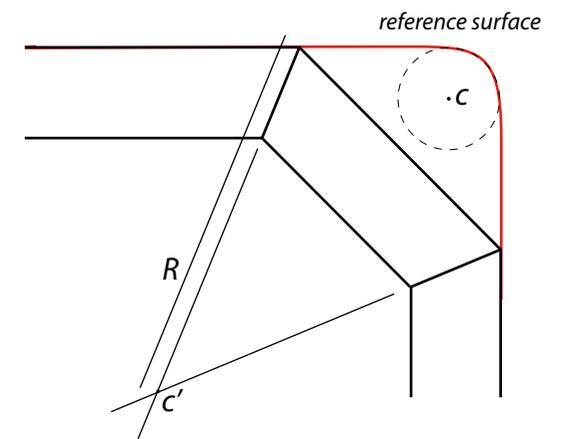
Figure 3.12 - relation between curvature radius element size and element thickness
