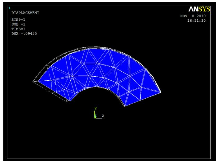
Figure 4.43 - Finite element analysis on deformation under vacuum pressure
