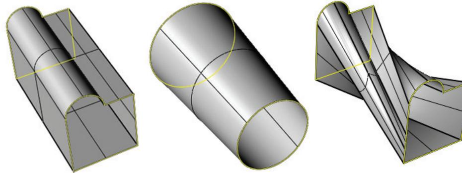
Figure 2.44 - extrusion, tapered loft and irregular surface (occurs when spindles have a different strating position)
