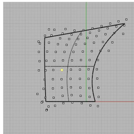
Triangulation based on maximum edge length. From one selected point a rectangular grid is draped over the surface, maintaining equal distances between points. This results in a more evenly spread division.
