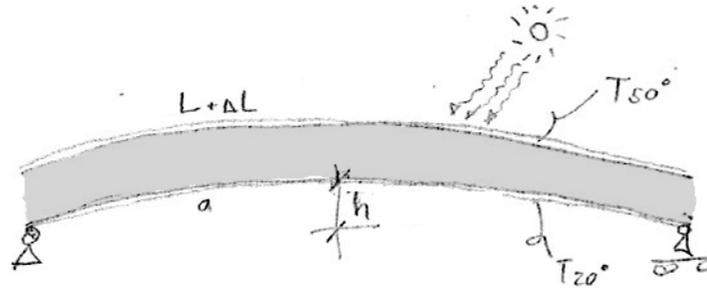
Figure 2.37 - Heat load by solar radiation
