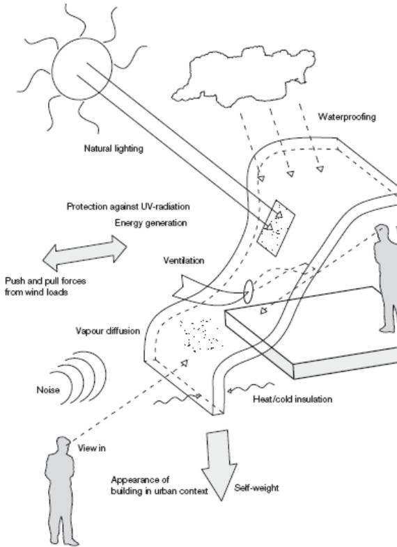
Figure 2.21 - functions of a facade (Knaack, 2006)
