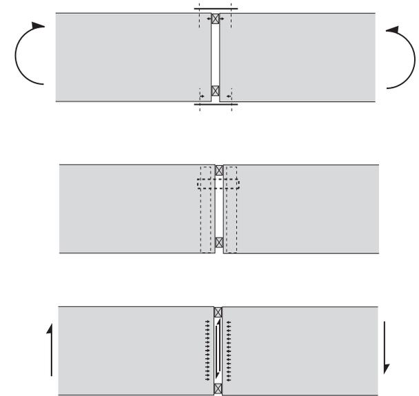
Figure 3.16 - internal forces in rigid connection
