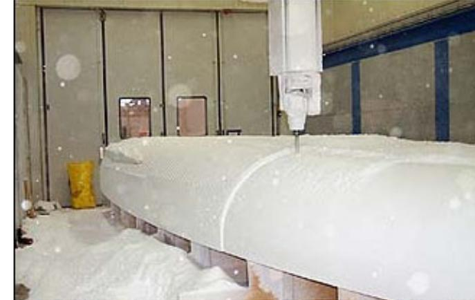
EPS blocks were CNC milled and put together on site. EPS was covered in protective film to prevent styrene released in hardening process of polyester to solve the EPS. Face is applied in manual lamination process, using slurry of resin and fibres.
