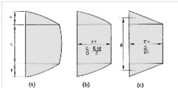
Figure 2.27 - shear force equal distributed over the height when faces are thin (c)
