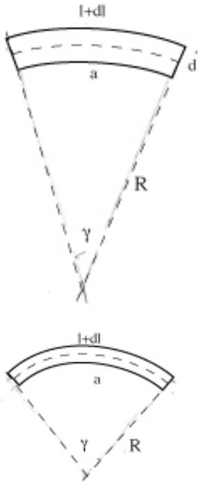
Figure 2.38 - curvature increases if top face expands
