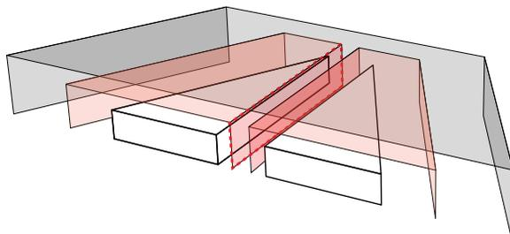
Figure 3.31 - separate core elements are covered in glass fabric to construct shear web (red)
