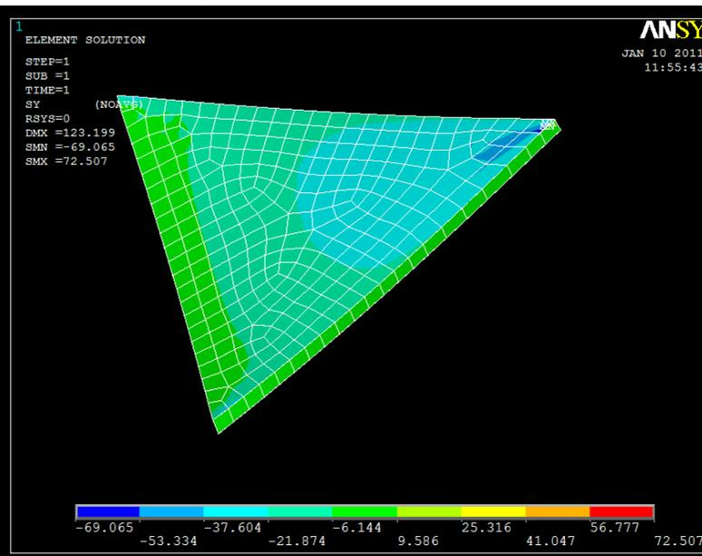
7. normal stress with layer thickness 5-500-4mm
