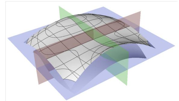
Figure 3.4 - division by orthogonal projection
