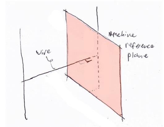
Figure 4.41 - reference plane perpendicular to initial wire position
