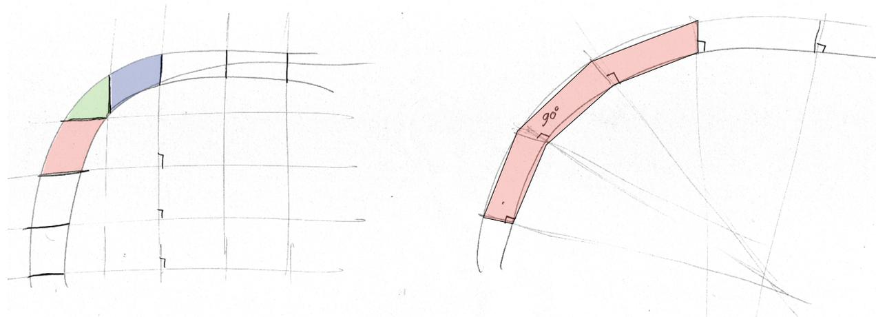
Figure 3.8 - uniformity of elements, right orthogonal, left triangulation
