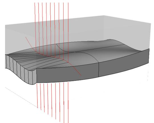
Figure 3.5 - Layered object manufacturing (LOM)
