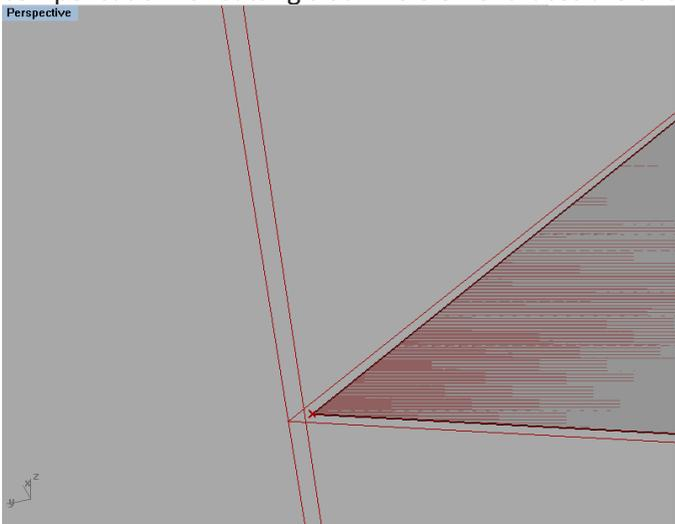
Corner points are connected and projected to two planes perpendicular to the base of the element, forming the coordinate points for the CNC spindles to move to.
