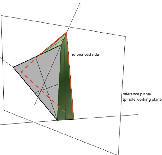
Figure 3.7 - referenced faces when raw material is placed against a reference plane in the cutting machine
