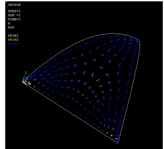
Figure 4.35 - Principal stress trajectories show stresses get diverted to the corners.
