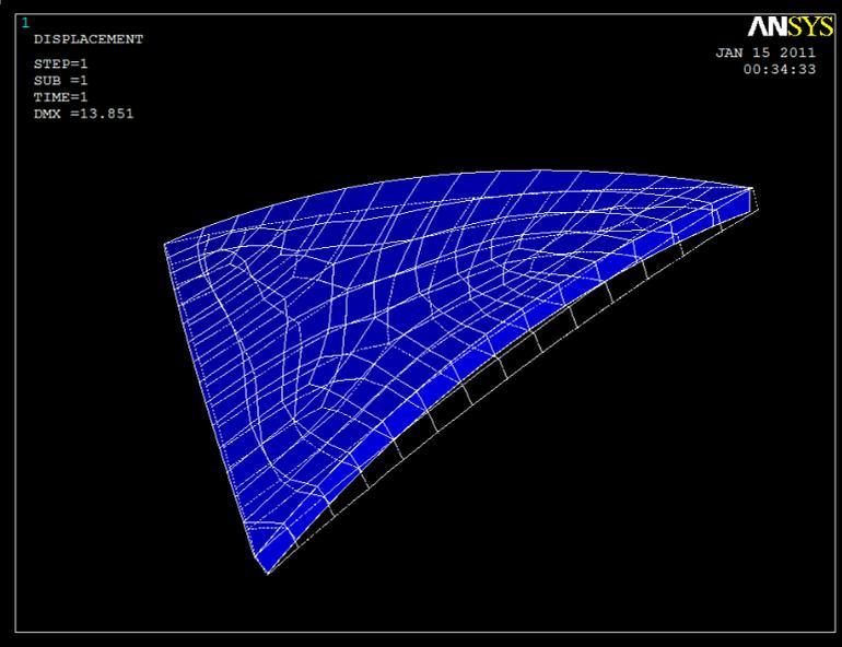
3. deflection caused by live load without safety factors (1,0kN/m2)
