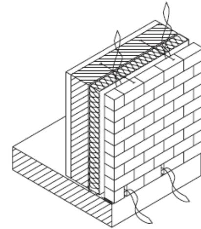
Figure 1.19 - functional layers of a facade
