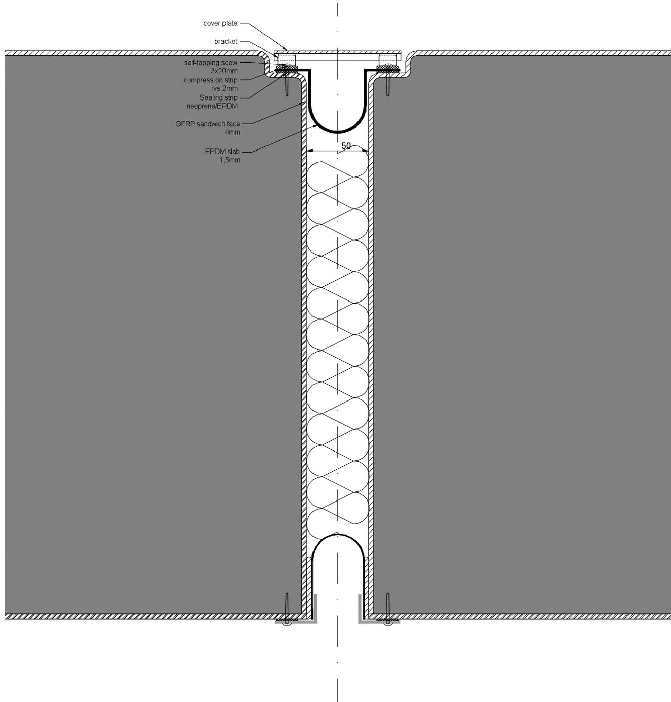
Figure 3.22 - final design expansion joint
