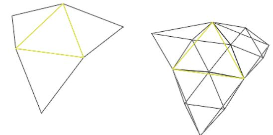
Figure 3.10 - refinement by splitting mesh and moving vertices to reference surface
