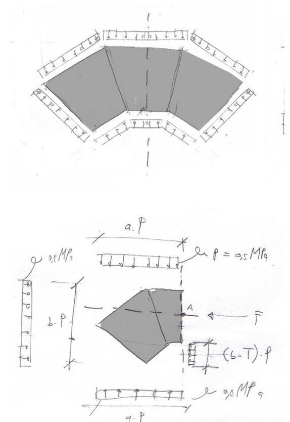
Figure 2.46 - vacuum pressure acting on the foam core of an injected sandwich element.
