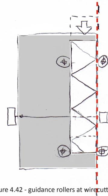
Figure 4.42 - guidance rollers at wire cutting machine
