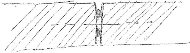
The butt joint with compressed seals is a simple solution. The sides of two adjacent elements are placed against each other. Seals are placed in between and the elements are pulled towards each other by a connecting element.
