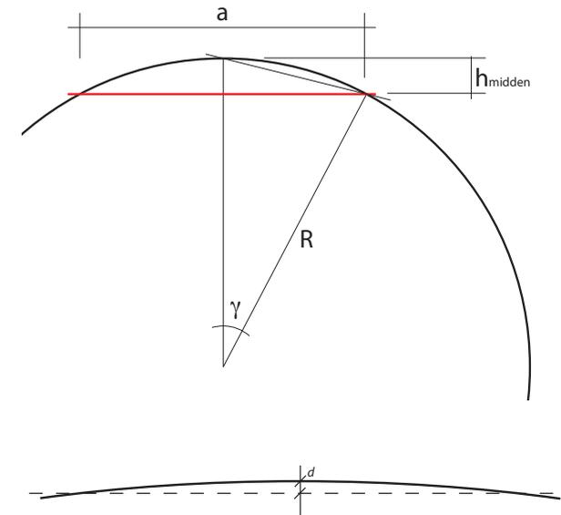
Figure 2.25 - curvature expressed in radius and deviation d
