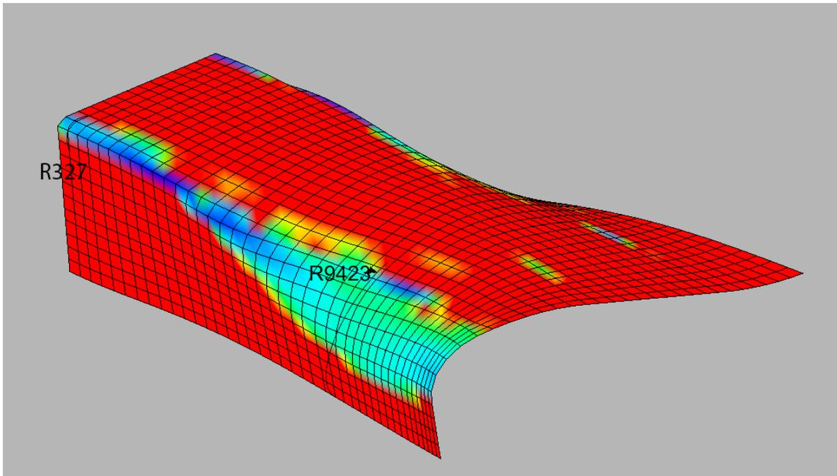
Figure 2.24 - curvature analysis, range blue - red represents curvatures from resp. 327mm to 20000mm in radius
