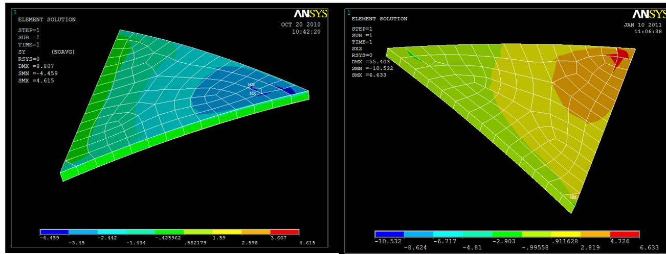
Figure 4.34 - normal stresses in the face and shear stress in x direction.
