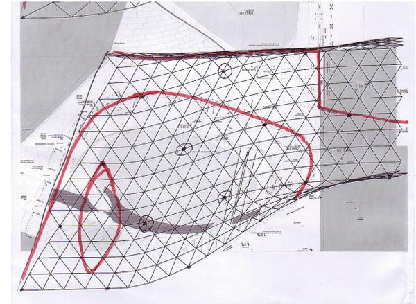
Figure 3.29 - floorplan of support positions
