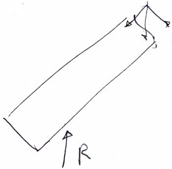
Figure 3.28 - shear forced decomposed when sandwich element is in an inclined configuration
