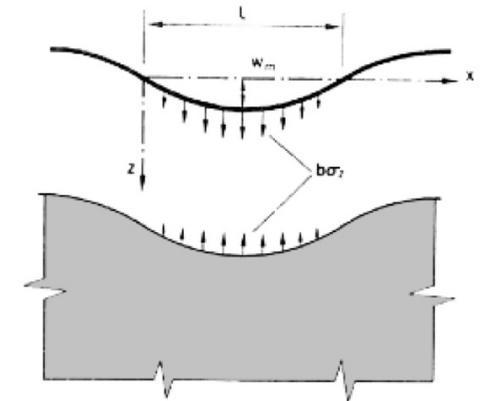
Figure 2.30 - sinusoidal buckling of the face, counteracted by elastic medium
