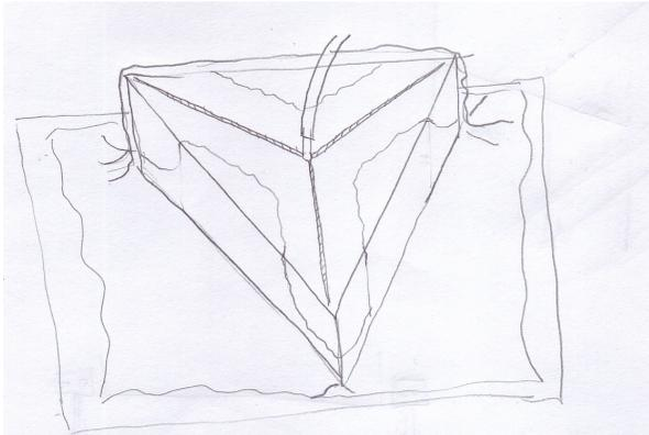
Figure 3.30 - vacuum bag, runners applied from the centre to the corners for improving resin distribution
