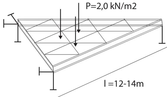
Figure 4.33 - loadcase for roof segments
