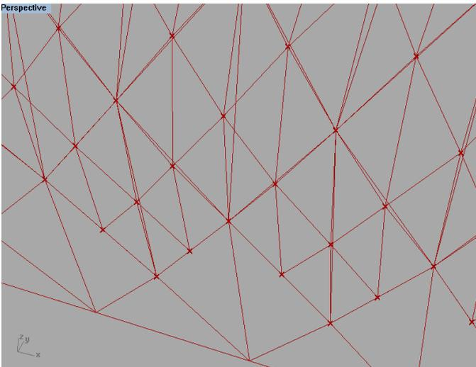
4 new triangles are formed from the 3 initial corner points and the new points projected on the reference surface.
