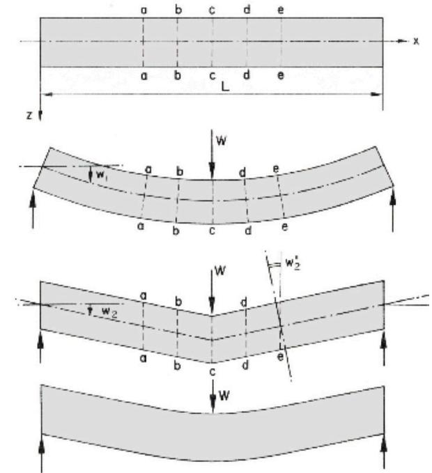
Figure 2.26 - shear and bending deformation
