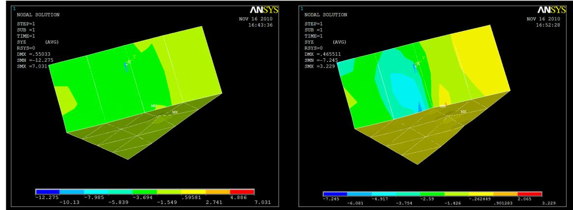
Shear stress is concentrated in three points instead of one, resulting in a better stress distribution. Peak stress did not decrease significantly by placing one support inwards from the corner. This is caused by the absence of a core material in the model, that would have better distributed the stress.
