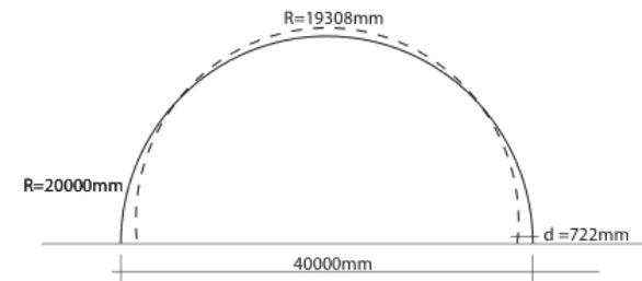
Figure 2.40 - theoretic curvature with circular span of 40000mm
