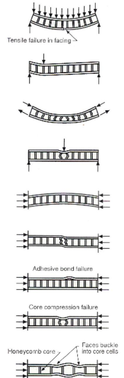
Figure 2.32 - failure types
