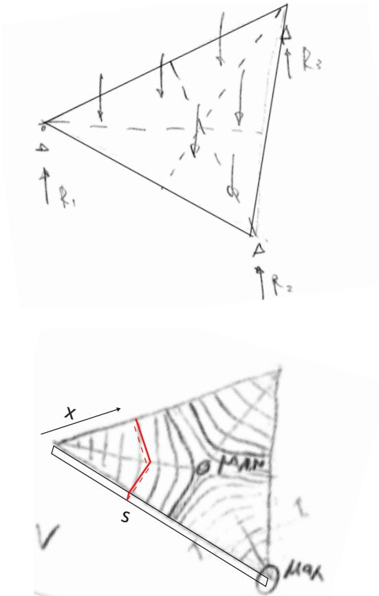
Figure 2.35 - Shear force peaks occur near the supports and is zero in the lines equidistant from the supports
