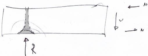
Figure 3.27 - shear webs reinforcement at the support. Bending moment at the connection (right side) occurs
