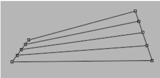
Figure 2.43 - ruled surface, points are at the same period at the opposite edge curves. Connecting them results in straight lines
