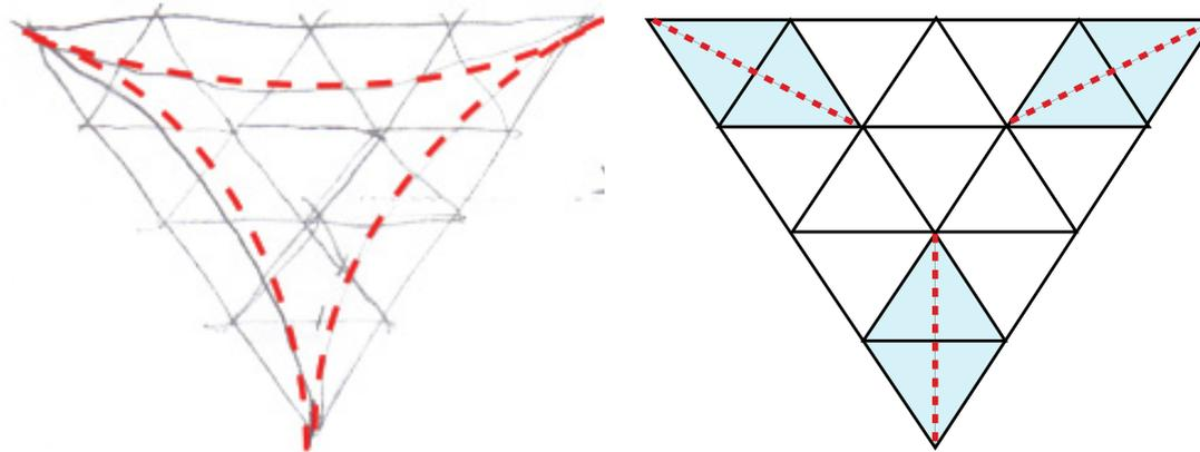
Figure 3.26 - locations for shear webs (red dotted lines)
