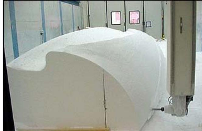
Figure 1.7 - milling of EPS blocks
