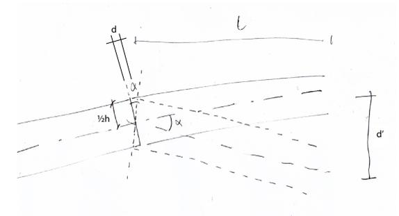
Figure 3.14 - inaccuracy in side can cause large deviations from the reference surface
