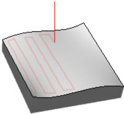
Figure 1.17 - CNC milling 3 dimensional path
