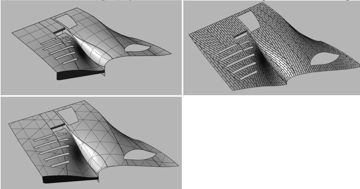
The segments are self-supporting over a span of 10 -16m, derived from the design aspects. The segments are subdivided in smaller elements.
