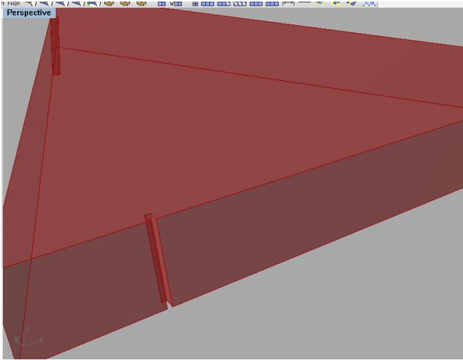
Face borders are extended with extrusions and joined into one curve. Curve is offset in plane with variable threshold as a compensation for cutting slot. The element faces are offset
