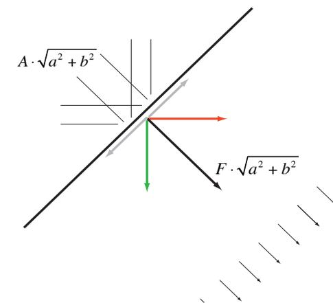
Figure 2.33 - combined magnitude of two orthogonal force vectors on an inclined plane
