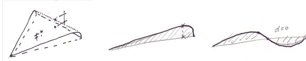
In the Arnhem context, the transport size limitation of 3m elements result in a fine enough mesh to exclude this problem. There are no wave patterns within the reference surface.
