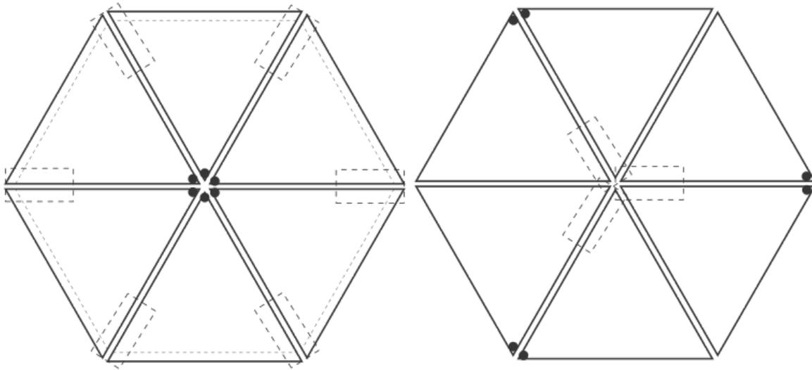
Figure 3.24 - support of roof segments, dots are fixed corners dotted lines represent supports with freedom of translation in one direction
