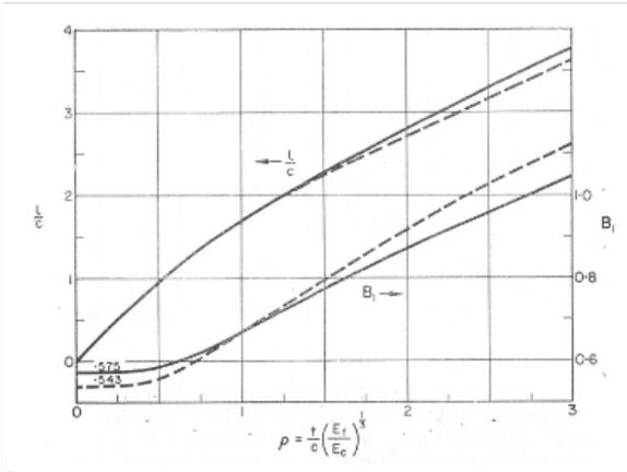
Figure 2.31 - Buckling constant  $B_1$  plotted against  $\rho$ , for most practical cases in building design  $\rho < 0,25$
