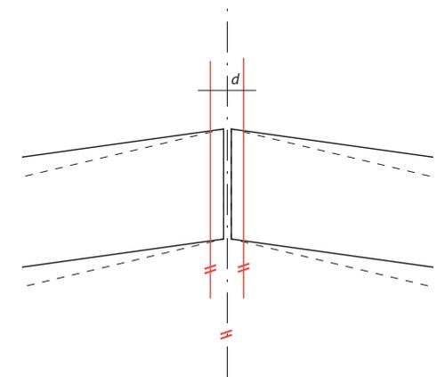
Figure 3.19 - Shape parameters used for referencing the fixture components.  $d$  is a fixed distance
