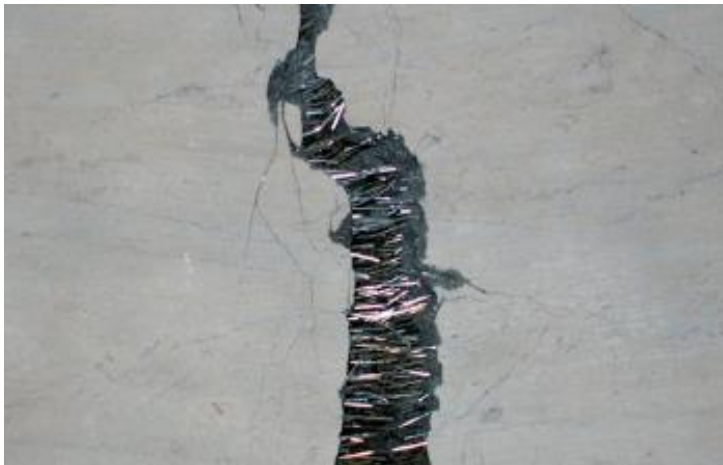
UHPFRC under a 4-point bending test
