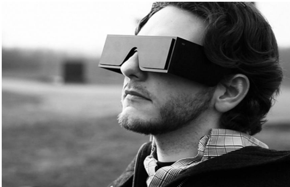
Figure 2-13. Picture of the prototype of Song of the machine by Superflux. It is an alternative remedy for visually impaired people. The patient’s nerve cells are inoculated with new genes. After that, the patient will wear a device that interprets the visual scene and sends coded pulses to the brain, enhancing the visual experience (Pavlus, 2011). Source: Superflux webpage.
