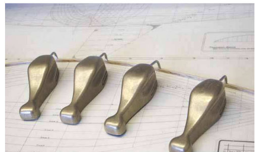
Fig. 5: Splines used e.g. for ship design
