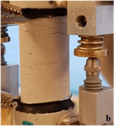
Figure 7.4: Multiple cracks developed during tensile test.
