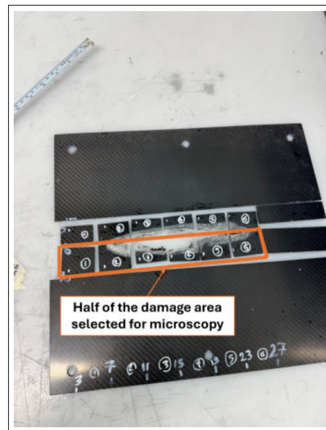
(c) Composite plate after cutting, V22
