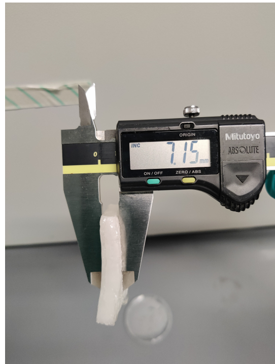
(b) Shrunken 40mm square thickness.
