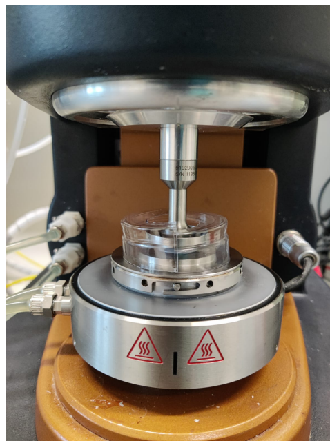
Figure 4.7: Rheometer setup with solvent trap.
