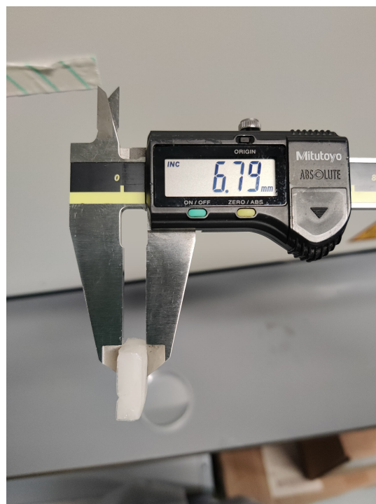
(b) Shrunken 20mm square thickness.
