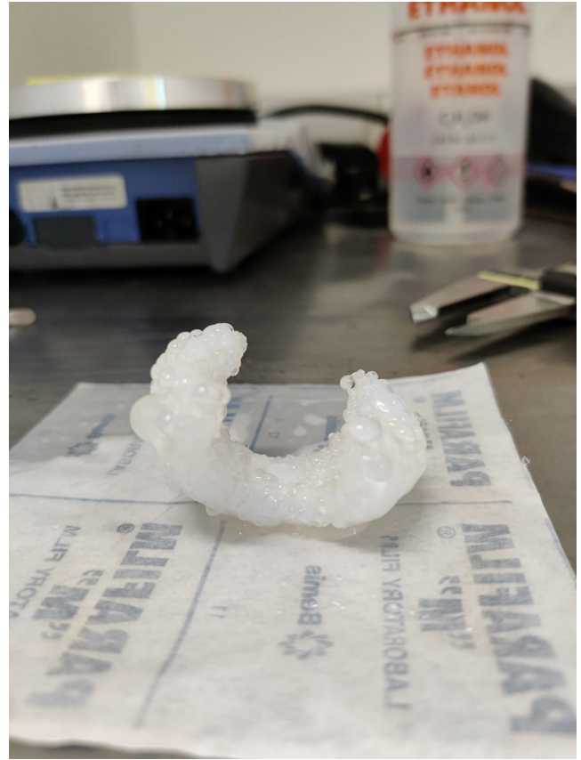
Fig. 20. Shrunken and deformed bow-tie shaped hydrogel.
