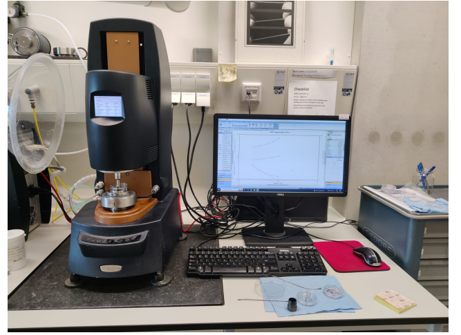
Fig. 2. TA Instruments Discovery HR-3 Rheometer test setup.
