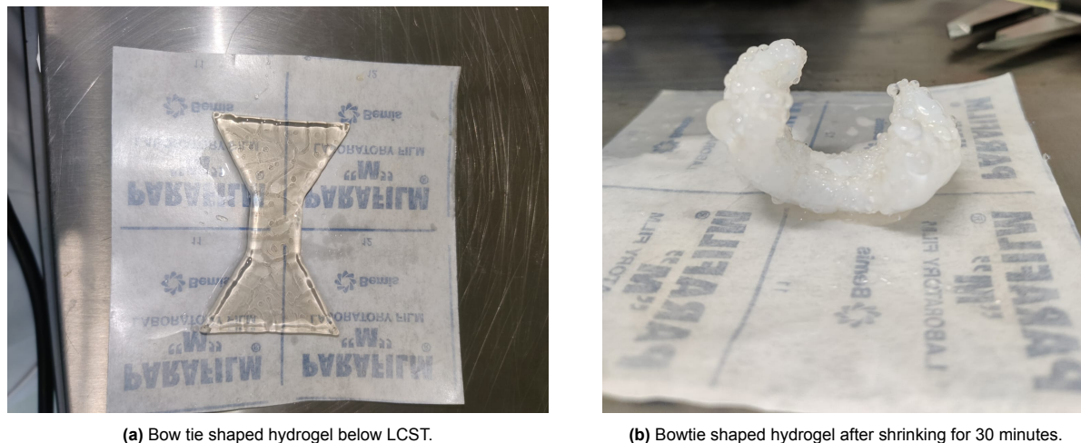
Figure 5.20: Bowtie shaped hydrogel before and after shrinking.
