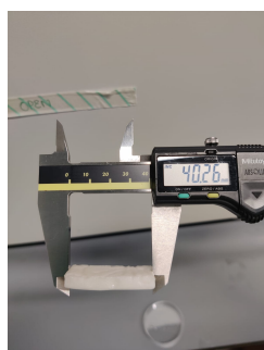
(a) Shrunken 40mm rectangular slab length.
