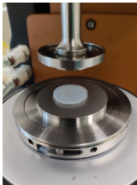
Figure 4.9: Hydrogel sample above LCST.
