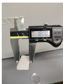
(b) Shrunken 40mm rectangular slab width.
