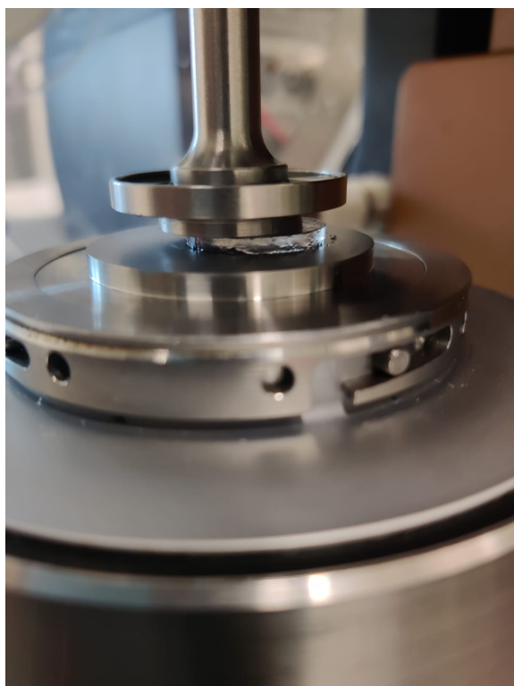
(a) Hydrogel slipping at higher strains.
