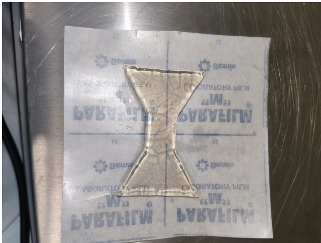
Fig. 19. Swollen bow-tie shaped hydrogel.
