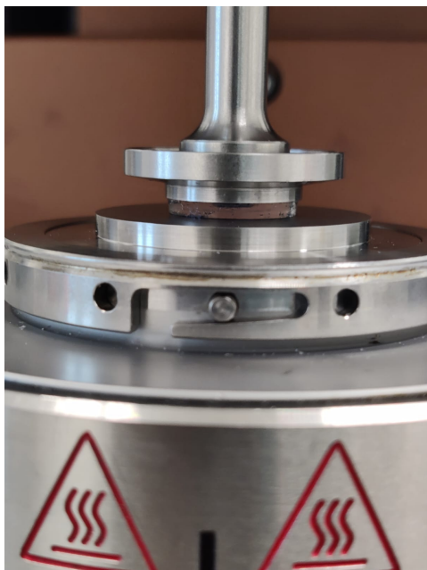
Figure 4.10: Below LCST loaded sample.
