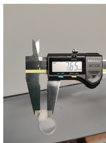
(c) Shrunken 20mm rectangle thickness.
