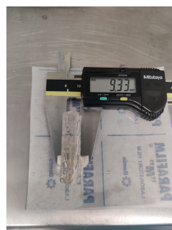
(f) Swollen 40mm rectangular slab thickness.
