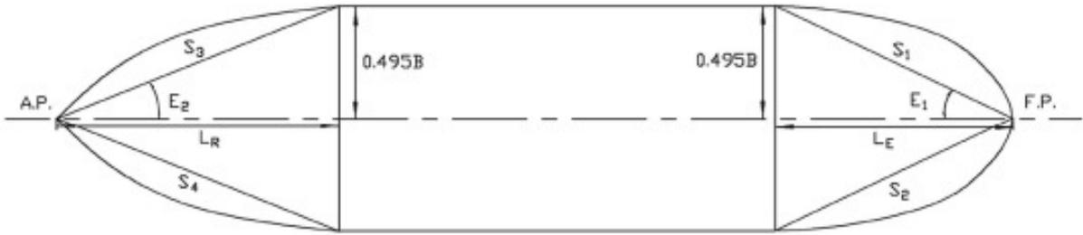
Figure 2.11: Segment and parameters definition
