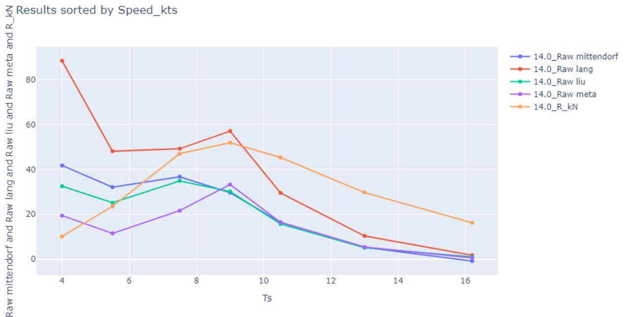
Figure 2.20: Wave added resistance, V=14kn, head waves, all models plus external data without first point
