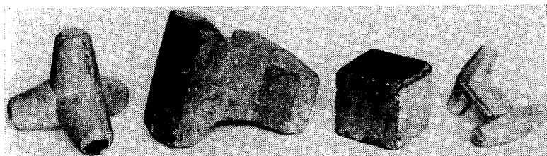
Fig. 5.1.b Tetrapod, akmon, cube, and dolos.
