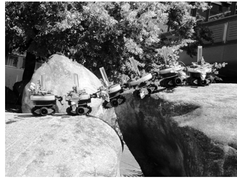
(b) Swarm-bots forming a chain to bridge a gap, which is too large for an individual to cross alone. The SWARM-BOT project develops hardware for testing and using the capability of self-assembling, self-organizing, and metamorphosis of robotic systems at ULB, Brussels, Belgium and EPFL, Lausanne, Switzerland. © LIS, EPFL. Reprinted with permission.
