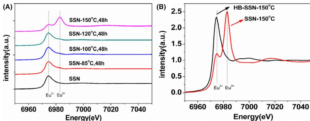
FIGURE 5 Normalized Eu  $L_{III}$ -edge XAFS of (A) SSN phosphors, as-prepared and after thermal treatment at different temperatures (for 48 hour), and (B) comparison of the corresponding plots for SSN and HB-SSN after thermal treatment at 150°C [Color figure can be viewed at [wileyonlinelibrary.com](http://wileyonlinelibrary.com)]
