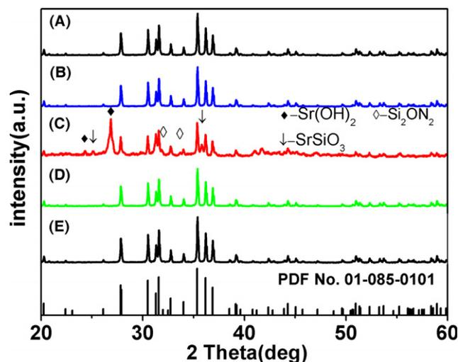
**FIGURE 3** X-ray diffractograms of SSN (A: as-prepared, B: treated at 120°C, C: treated at 150°C), and HB-SSN (D: as-prepared, E: treated at 150°C). The diffraction patterns SSN (JCPD No. 36-0570) are also plotted [Color figure can be viewed at [wileyonlinelibrary.com](http://wileyonlinelibrary.com)]
