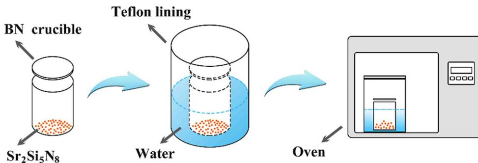
FIGURE 1 Moisture-induced degradation experiment [Color figure can be viewed at wileyonlinelibrary.com]
