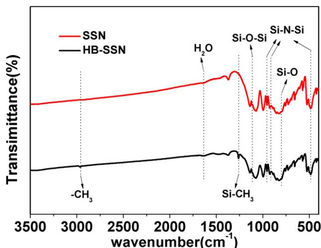
FIGURE 6 FT-IR spectra of SSN and HB-SSN [Color figure can be viewed at [wileyonlinelibrary.com](http://wileyonlinelibrary.com)]
