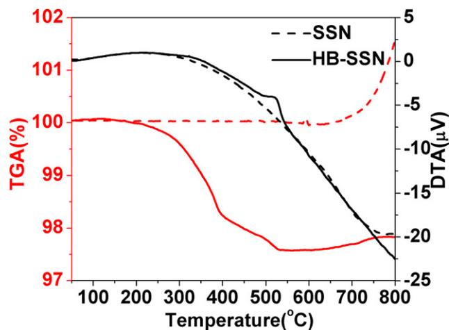
**FIGURE 9** Thermal analysis (TGA and DTA curves) of SSN and HB-SSN in air atmosphere [Color figure can be viewed at wileyonlinelibrary.com]
