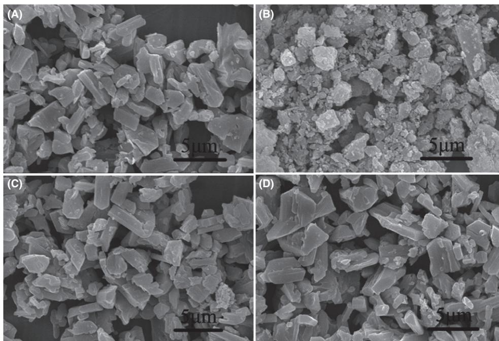
**FIGURE 4** SEM images of SSN (A: as-prepared, B: treated at 150°C), and HB-SSN (C: as-prepared, D: treated at 150°C).
