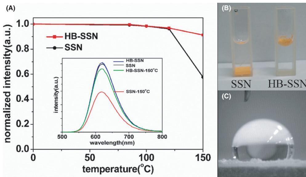
FIGURE 2 A, Emission intensity excited at 425 nm of SSN and HB-SSN treated with water steam at different temperatures for 48 hour (the inset shows the photoluminescence spectra); B, photographs of SSN and HB-SSN powders in water; C, contact angle of water drop on the surface of HB-SSN (at room temperature) [Color figure can be viewed at wileyonlinelibrary.com]
