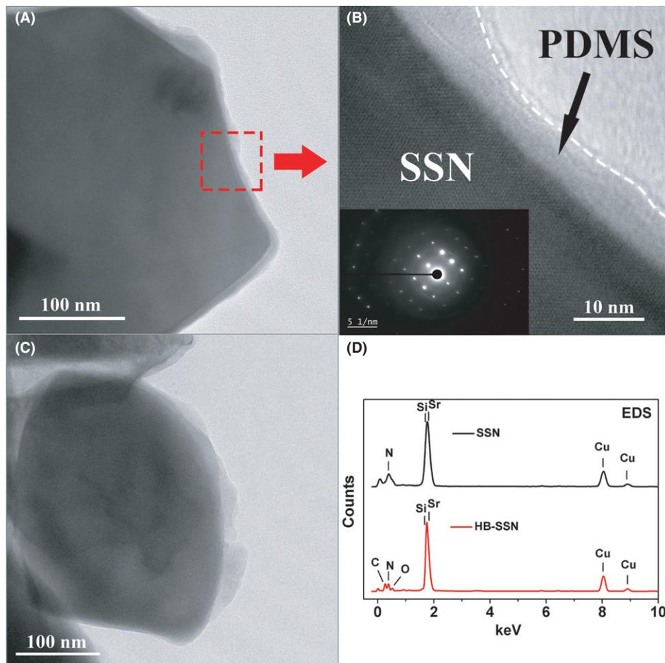
**FIGURE 7** TEM (A) and HRTEM (B) images of HB-SSN, TEM image of SSN (C), and EDS spectra from the surface of SSN and HB-SSN particles (D) [Color figure can be viewed at [wileyonlinelibrary.com](http://wileyonlinelibrary.com)]
