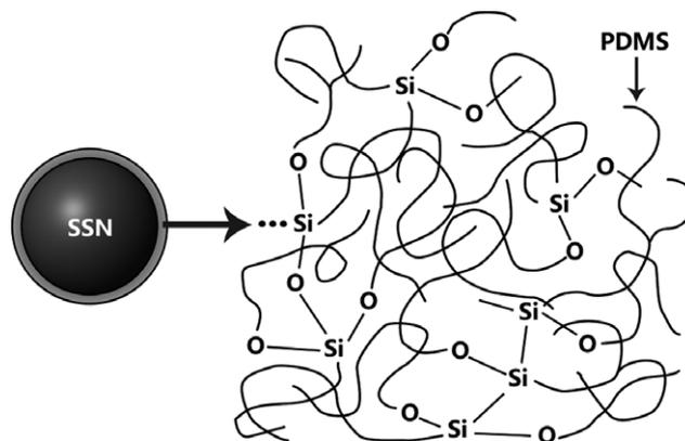
**FIGURE 8** A schematic drawing of the structure on the surface of the SSN particle
